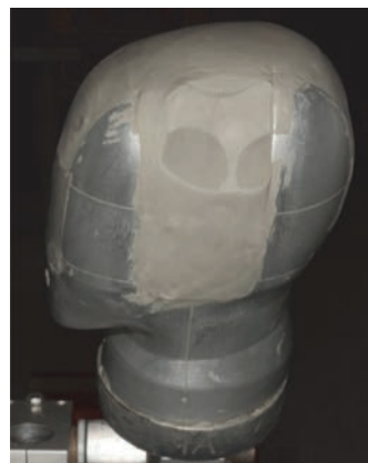
National Institute of Justice (NIJ) Back Face Deformation (BFD) Headform
