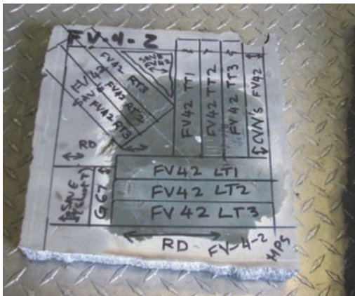
Test Specimen Cut from Amphibious Assault Vehicle (AAV) Hull
