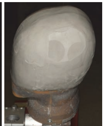
Peepsite Generation 2 (PG2) Back Face Deformation (BFD) Headform
