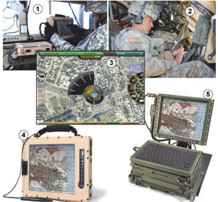
1 - JBC-P on Mounted Family of Computer Systems (MFOCS) 2 - JBC-P on Joint Version - 5 (JV-5) Block 2 3 - JBC-P Screen Shot 4 - JBC-P LOG on Military Rugged Tablet Plus (MRT+) 5 - JBC-P on JV-5 Block 2
