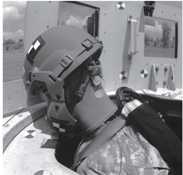
Helmet with Mandible Protection under Test
