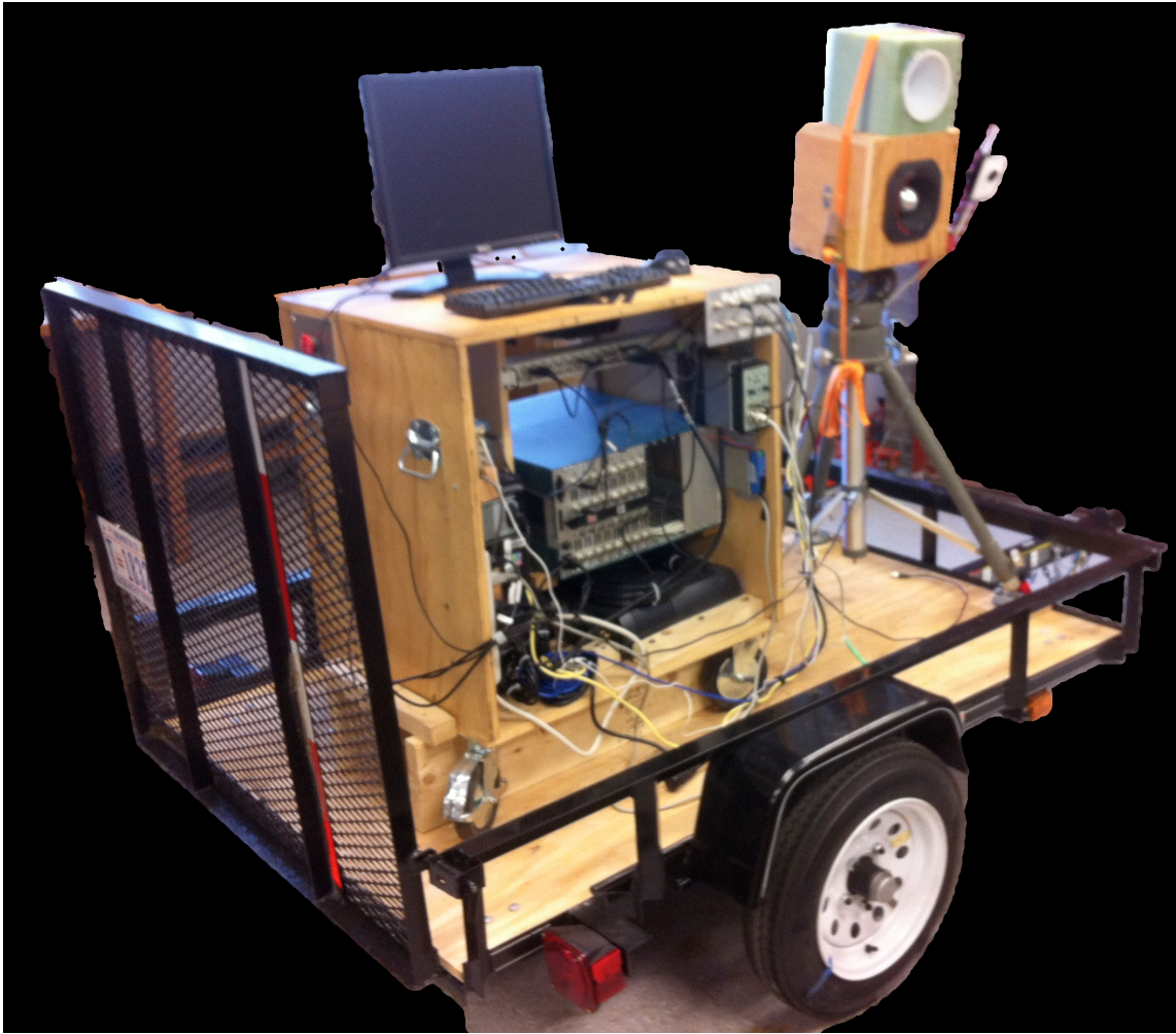
Figure 3.1: The first generation of the SAA field system used a desktop computer as non-specialized laboratory instrumentation.
