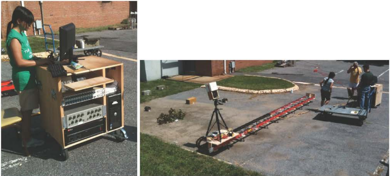
Figure 2.2: (left) The control station for the rail based system consists of a PC with a National Instruments data acquisitions system, audio filters and power amplifier and all other support electronics. (right) 5m rail mounted monostatic imaging system transmits and receives acoustic chirps (2-15kHz) to and from a collection of surface laid targets.
