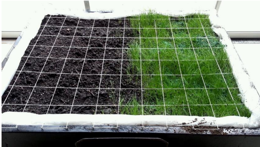
Figure 5.3: The sample grow box is show. On the right side is germinated Kentucky perennial grass. On the left side soil that has been sieved to 4.75 mm grain size. The 4 inch grid system marks each sample to be cut
