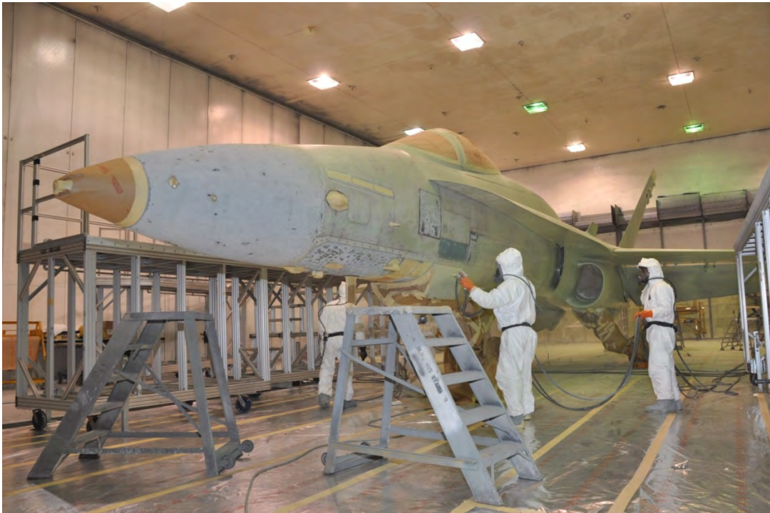
Figure 4: Photo of the refinishing of an F-18 aircraft in Bay 6 of Building 465 at Naval Base Coronado.
