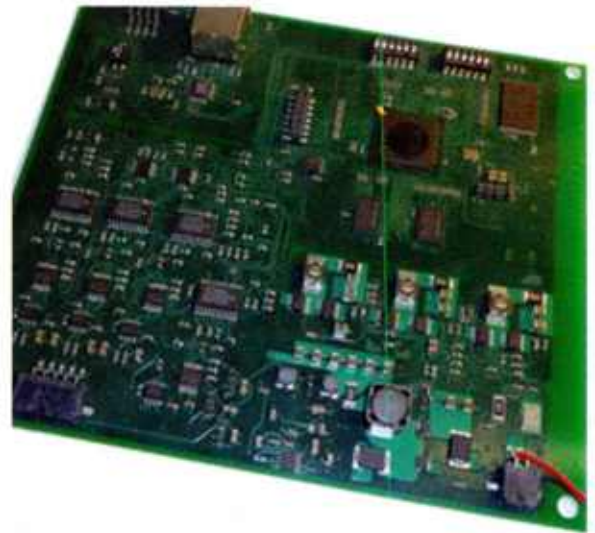
Figure 7. Vibration DAC Printed Circuit Board
