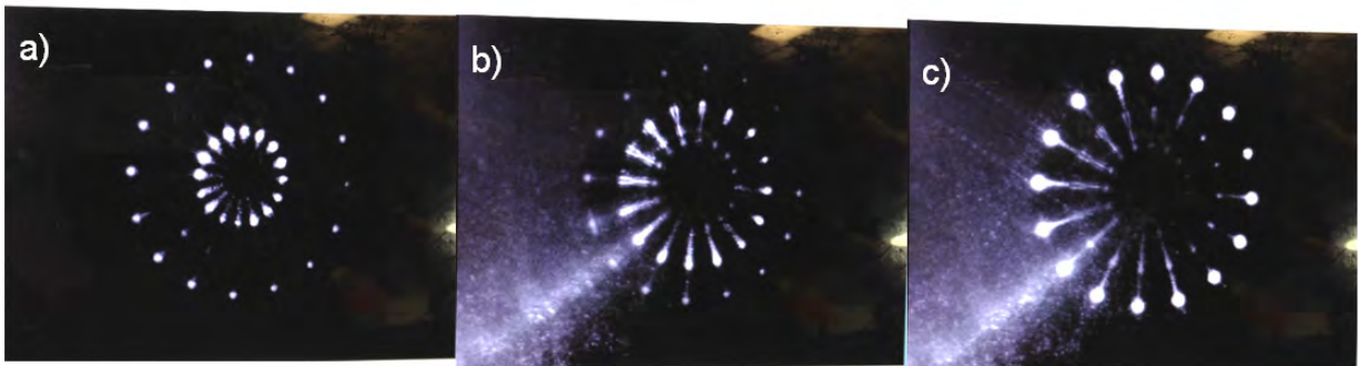
Figure 125. Grating emission of a) lowest layer b) middle layer c) top layer
