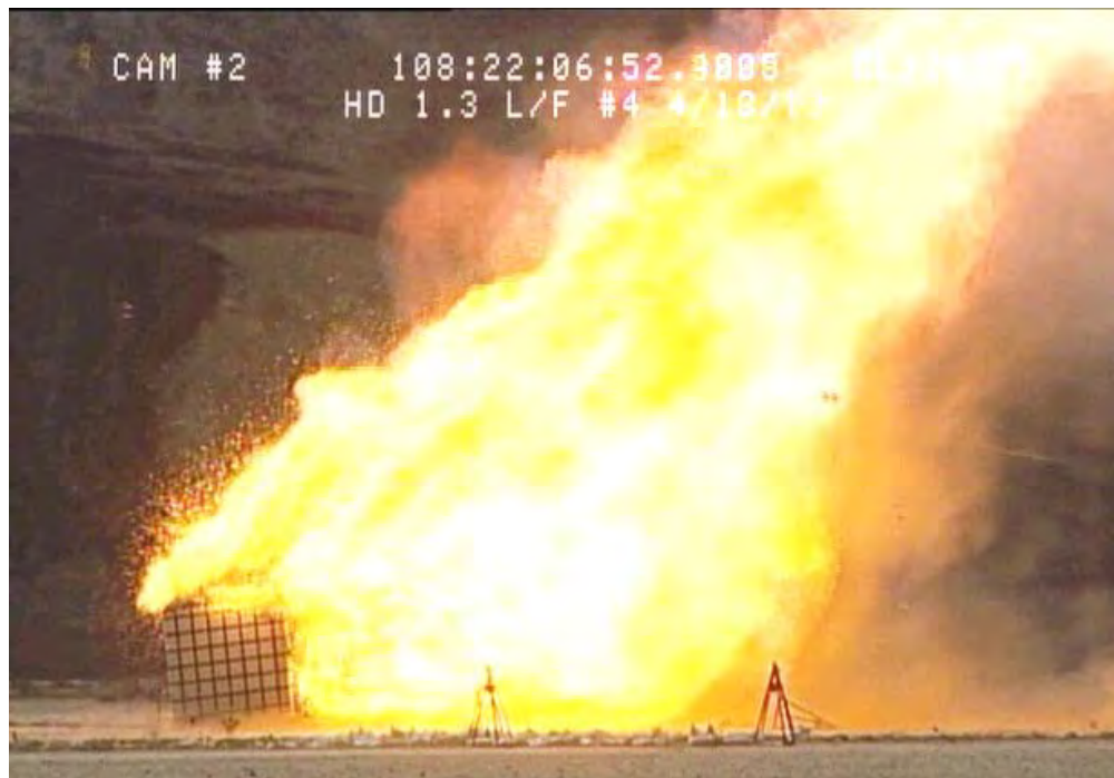
FIGURE I-20. Still Picture From Video Taken of Test 4 at 5 Seconds After Ignition (After Rupture of the Structure).
