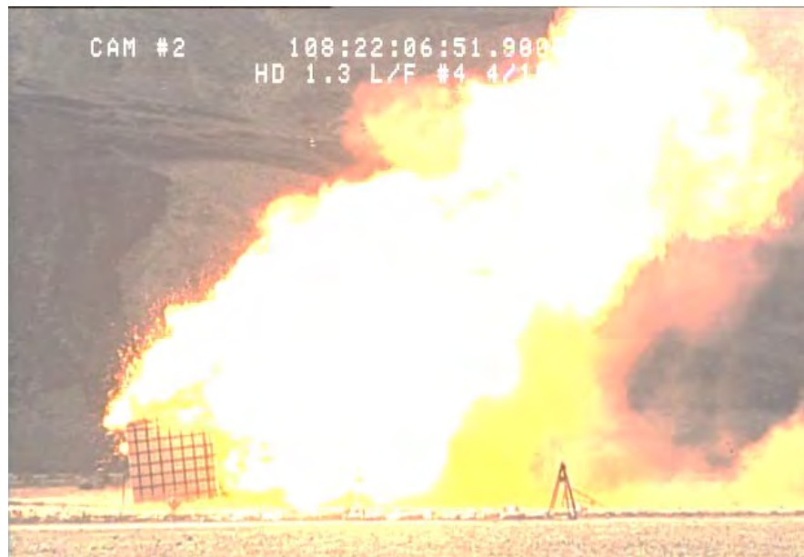
FIGURE V-19. Still Picture From Video of Test 4 at 4 Seconds After Ignition Showing Fireball From Ruptured Structure.
