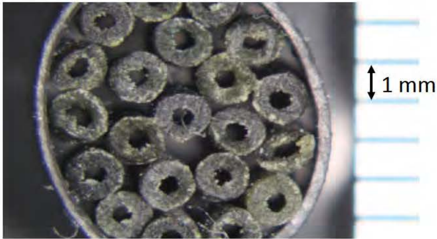
FIGURE I-2. End View of M1 Gun Propellant Grains Used in Tests 1 and 2.
