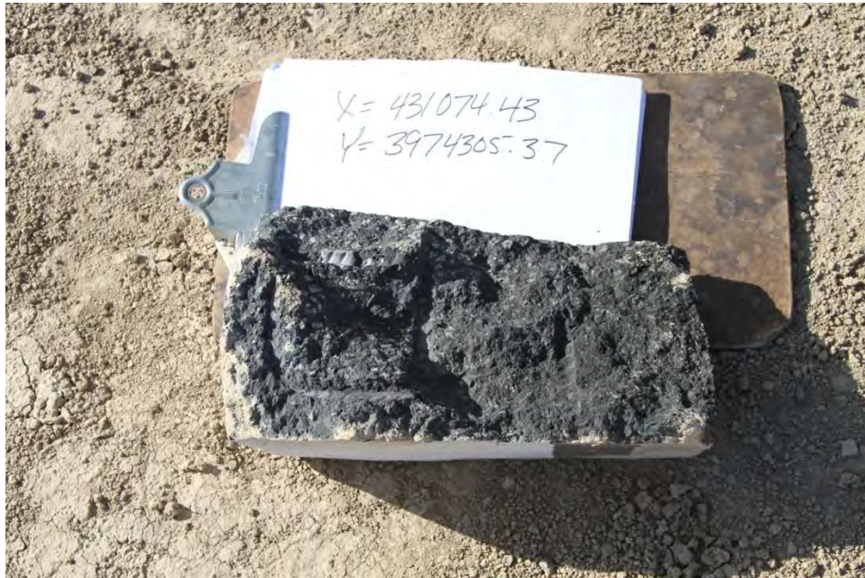
FIGURE V-G-3. Fragment From the Roof Weighing 8,790 g Found 22.2 m From Center of Original Structure (Test 4).
