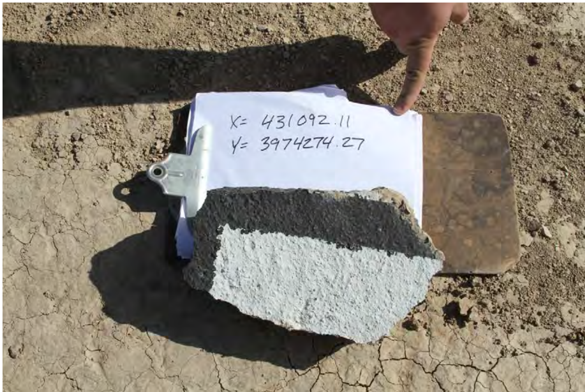
FIGURE V-49. Roof Fragment Weighing 4,535 Grams Found 25 Meters (82 Feet) FCOS (Test 4).
