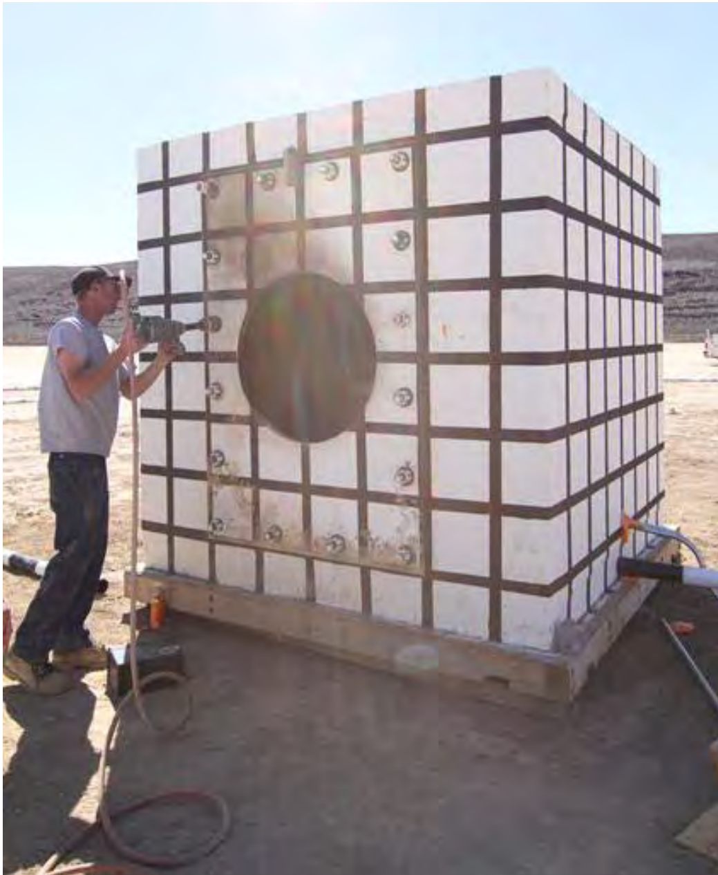
FIGURE I-7. Test Structure With Plate Having a 79-cm Orifice Bolted Into Place.
