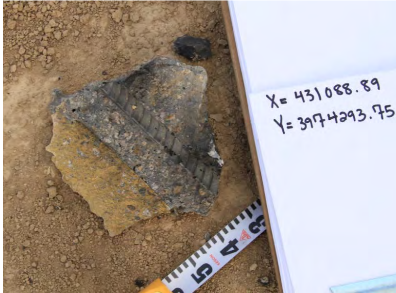
FIGURE III-G-26. Fragment From the East and North Wall Junction (Test 2). The fragment weight was 575 g and was found 7.6 m northeast from center of structure.
