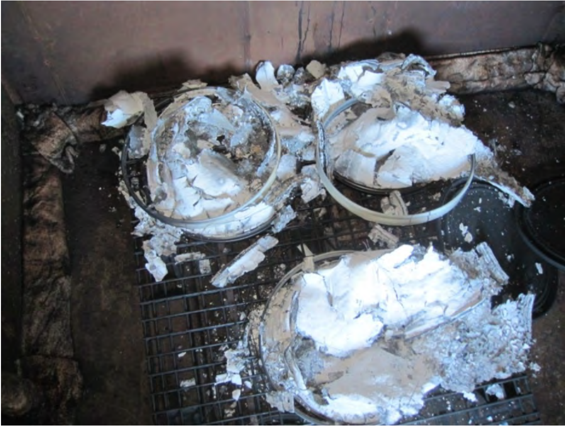
FIGURE II-7. Residue of Three Drums That Contained M1 Propellant in Test 1, 16 November 2012.
