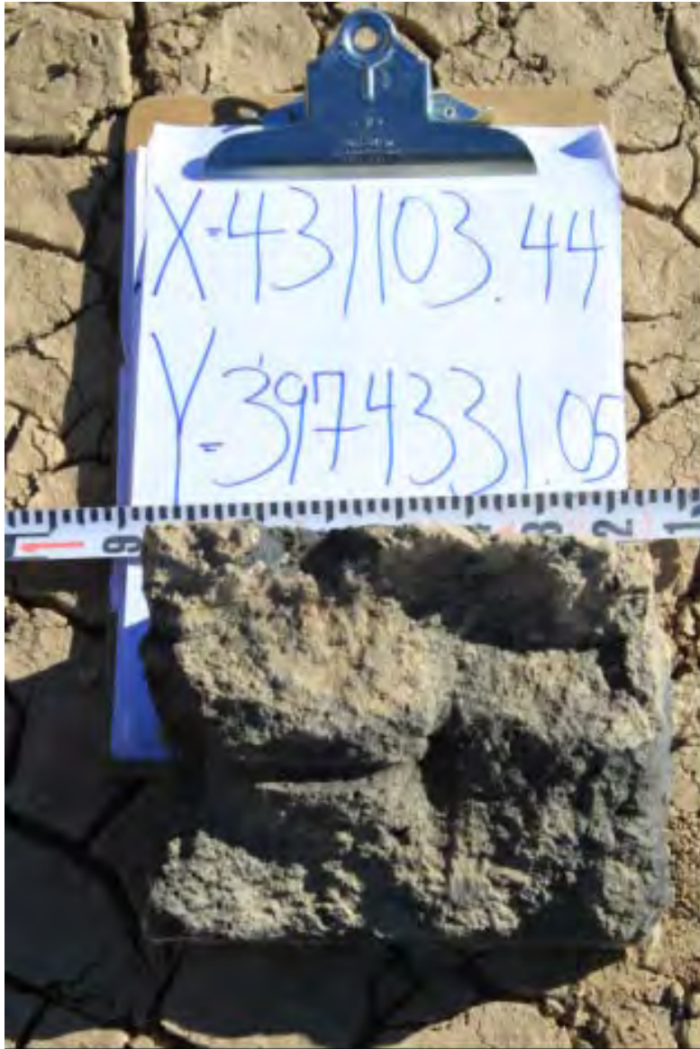
FIGURE III-G-12. Largest Fragment in the 4,000- to 4,999.9-g Weight Category at 4,958 g (Test 2) Found 40.5 m From the Center of the Original Structure Location.
