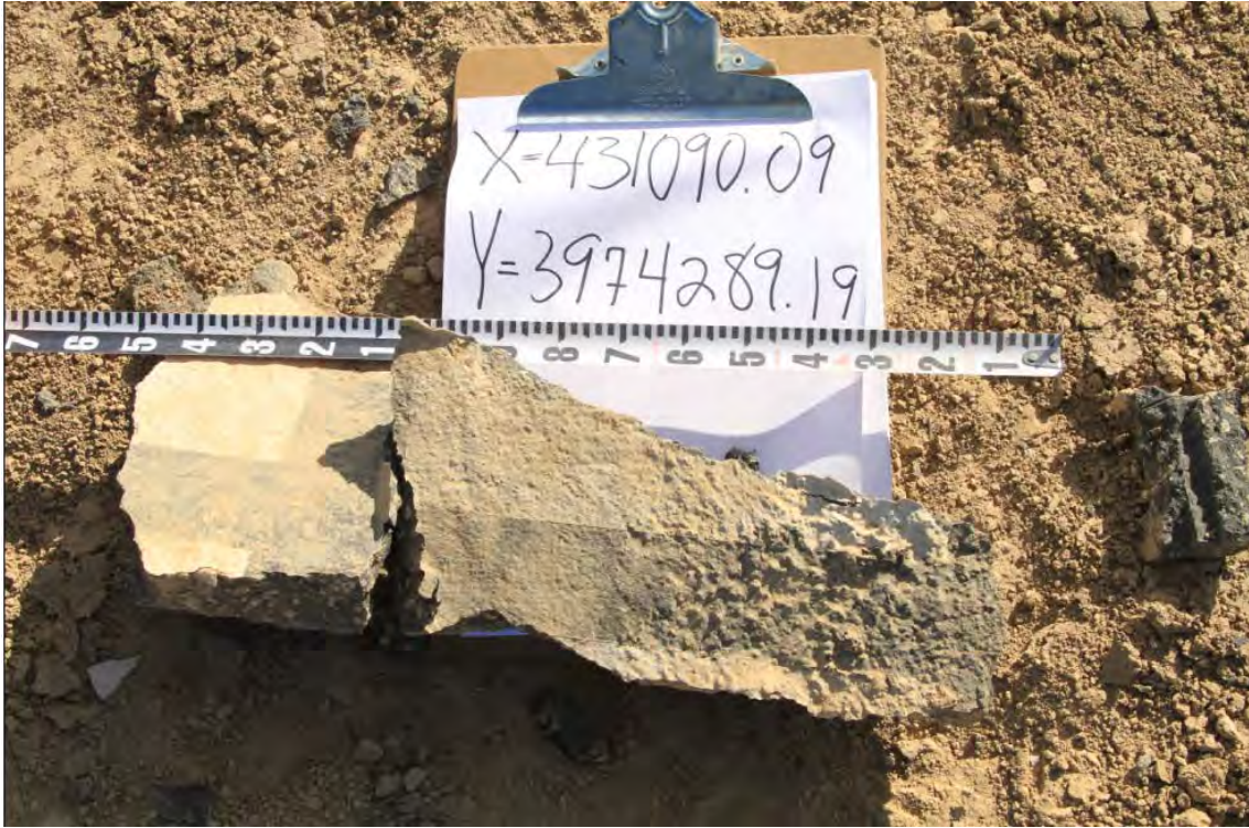
FIGURE III-G-10. Fragment Weighing 5,815 g Found 12 m South of the Structure (Test 2).
