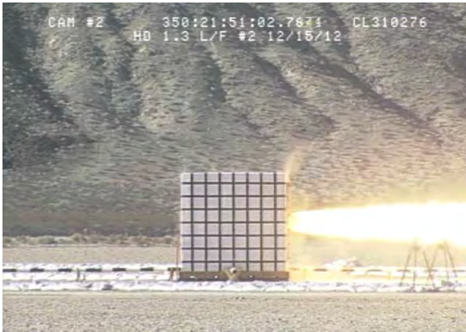
FIGURE III-16. Still Picture Taken From Video of Test 2 at 1.5 Seconds After Ignition. The plume is indicative of choked flow.
