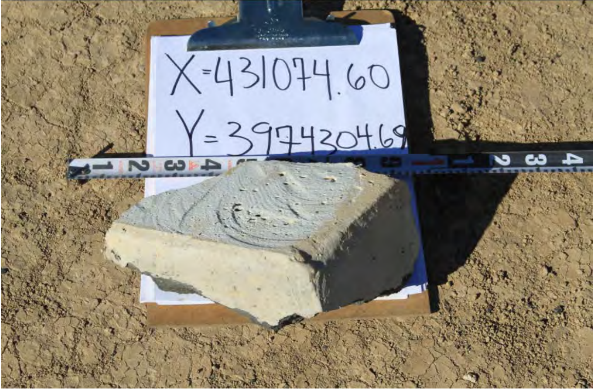
FIGURE III-G-18. Fragment That Originally had Been the Corner of the Roof, West Wall, and North Wall (Test 2). This fragment weighed 2,705 g.
