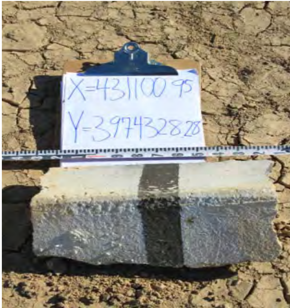
FIGURE III-G-2. Photograph of Largest Fragment (8,400 g) With Location Coordinates (Test 2).
