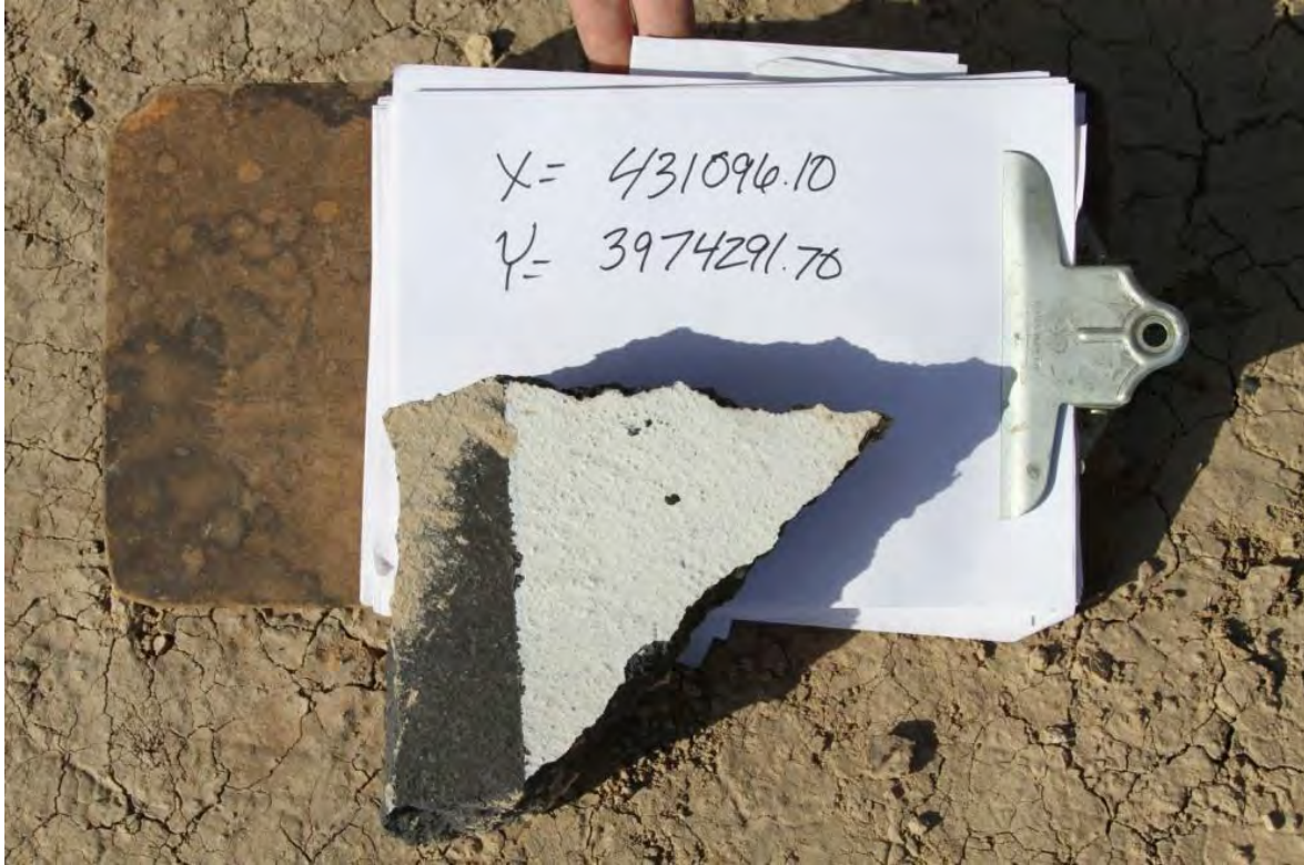
FIGURE V-G-18. Roof Fragment Weighing 2,025 g Found 13.8 m From the Center of the Structure (Test 4).
