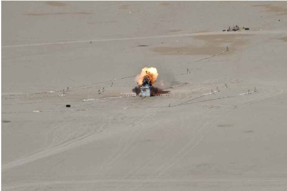
FIGURE V-15. Rupture of Roof, Fireball Formation and Debris Fragments Formed (Test 4).
