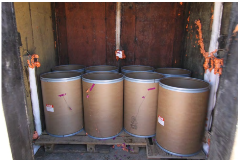
FIGURE V-1. Test 4 Structure With M1 Propellant Filled Barrels.
