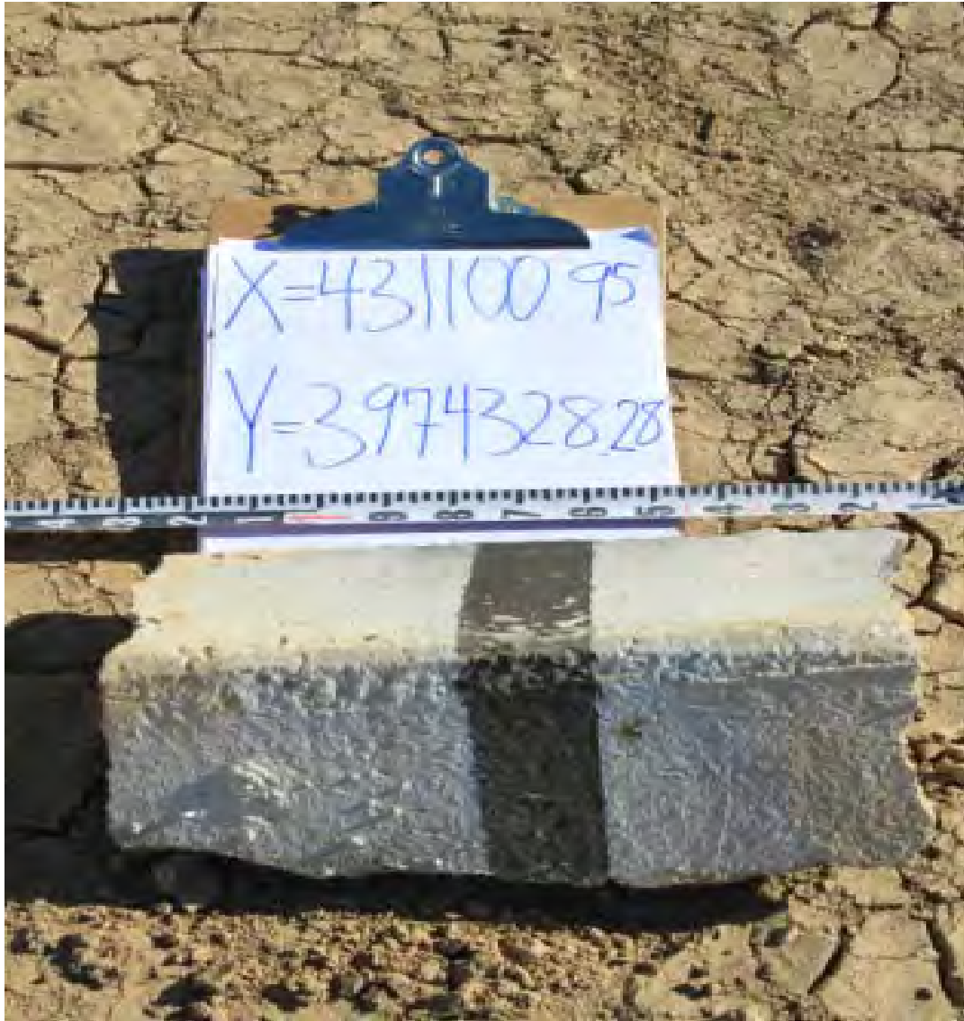
FIGURE III-36. Photograph of Largest Fragment (8,400 g) With Location Coordinates (Test 2).
