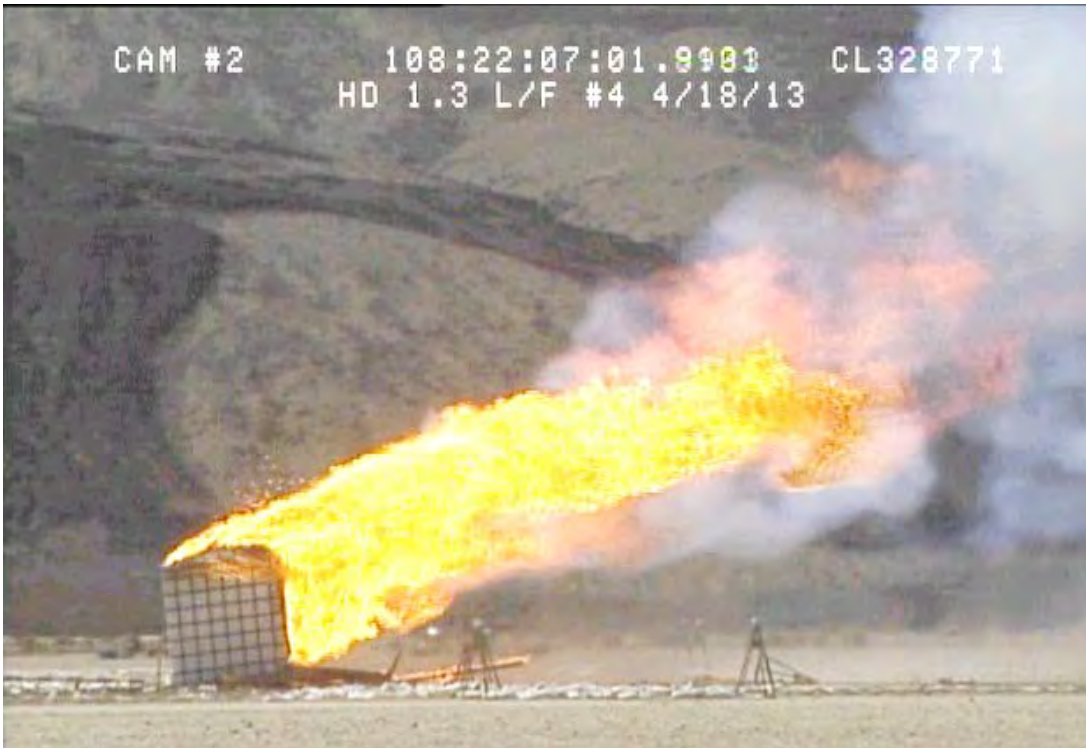
FIGURE V-23. Still Picture Taken From Video of Test 4 at 14 Seconds After Ignition.
