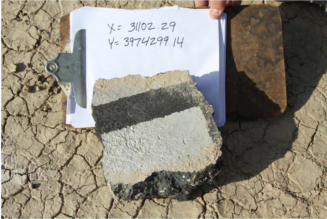
FIGURE V-G-13. Roof Fragment Weighing 4,390 g Found 3.5 m From Center of Structure (Test 4).
