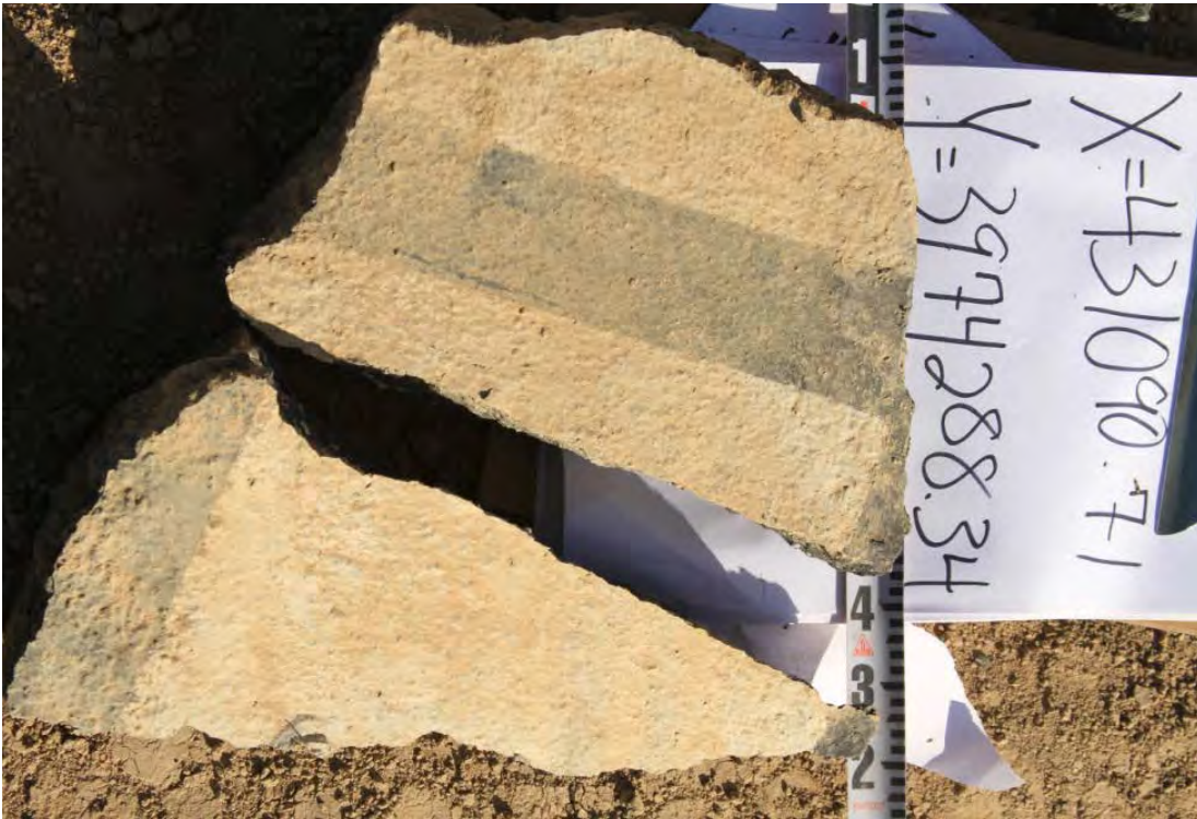
FIGURE III-G-6. Fragment Found to the Southwest of Structure With a Total Weight of 7,055 g (Test 2).
