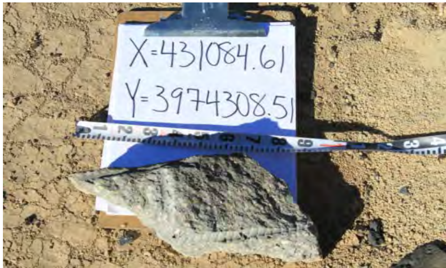
FIGURE III-39. Debris Fragment Weighing 2,605 g. This debris fragment shows both types of failure: rebar pulled through concrete obliterating the rib pattern (left) and fracture of the concrete from around the rebar preserving the rib pattern of the rebar.
