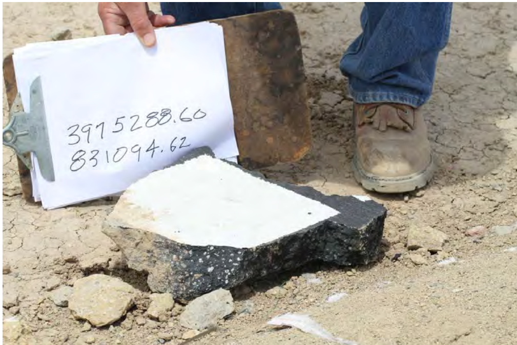
FIGURE V-45. Roof Fragment Weighing 8,740 Grams Found 14.25 Meters (46.8 Feet) FCOS (Test 4).
