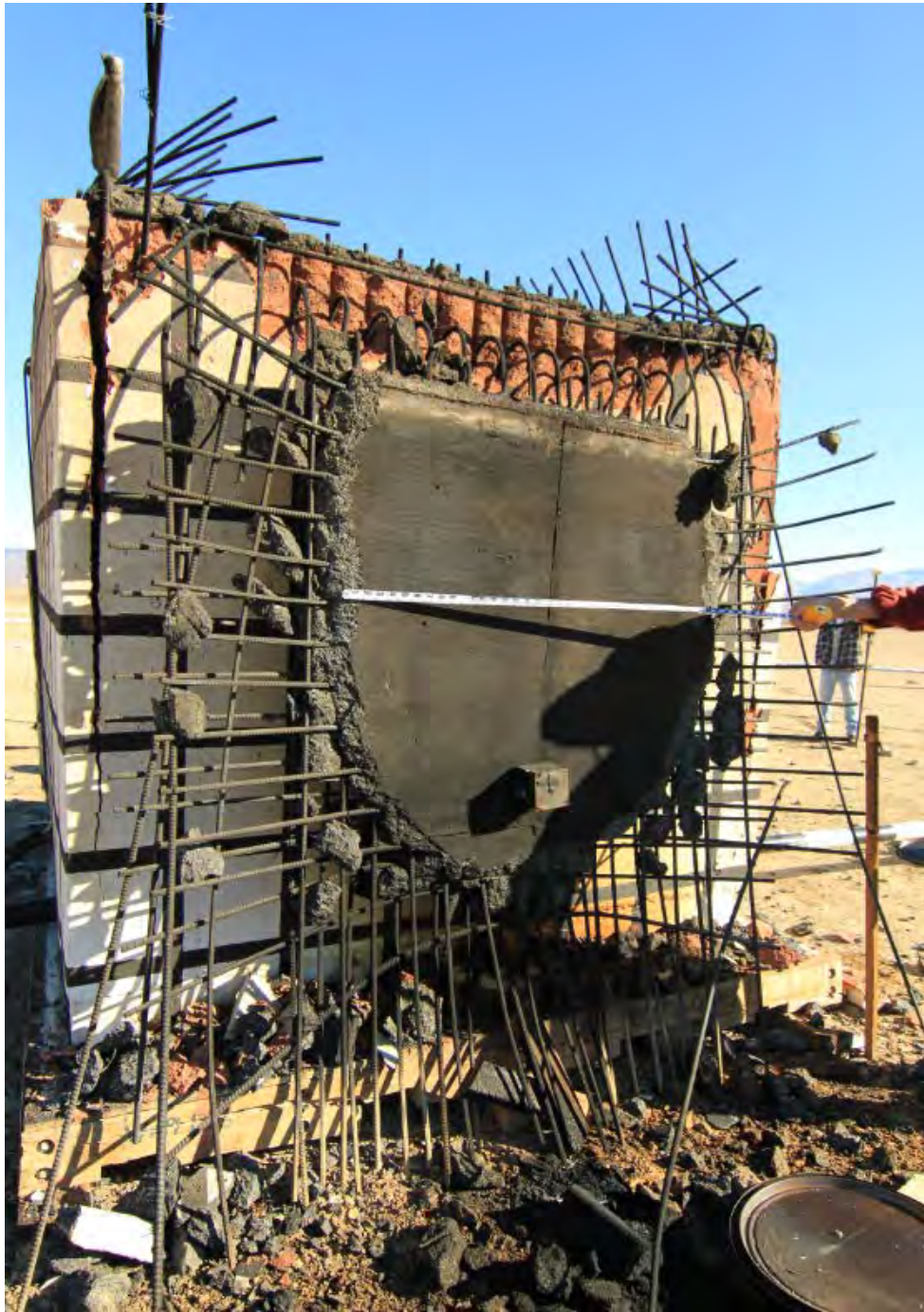
FIGURE III-26. What Was Left of Roof at Rest Against South Wall (Test 2).
