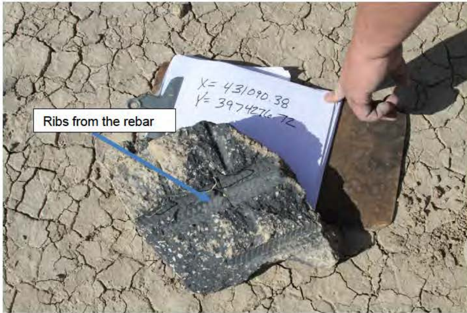
FIGURE V-46. Roof Fragment Weighing 6,375 Grams Found 22.2 Meters (72.8 Feet) FCOS (Test 4).
