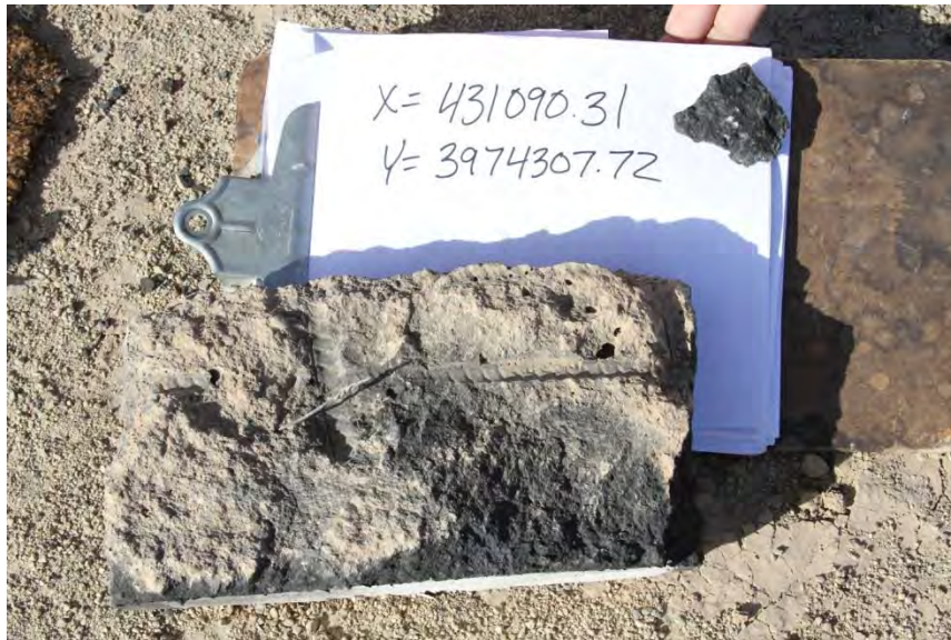
FIGURE V-G-9. Roof Fragment Weighing 6,325 g Found 11.8 m From Center of Structure (Test 4).
