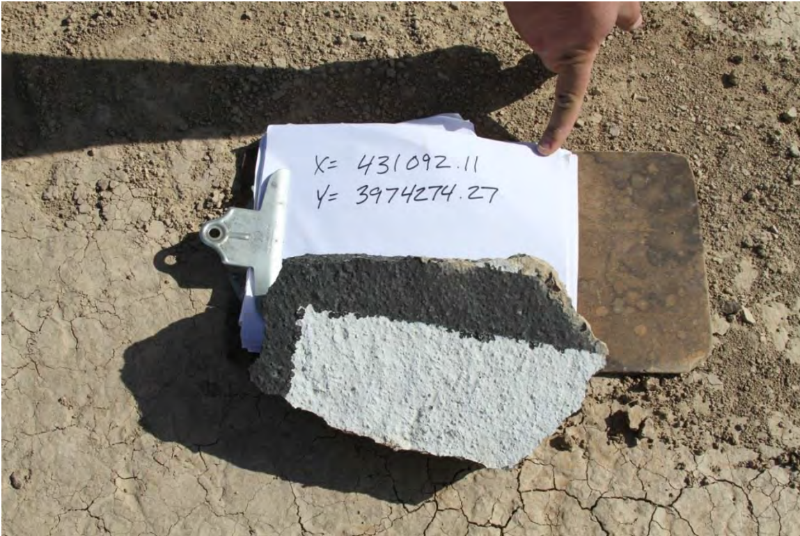
FIGURE V-G-12. Roof Fragment Weighing 4,535 g Found 25 m From Center of Structure (Test 4).
