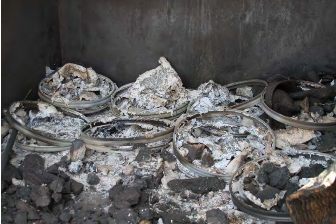
FIGURE V-10. Remains of Drums That Contained M1 Propellant (Test 4).
