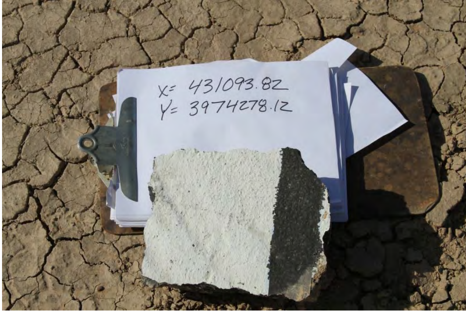
FIGURE V-G-15. Roof Fragment Weighing 3,905 g Found 22 m From the Center of the Structure (Test 4).
