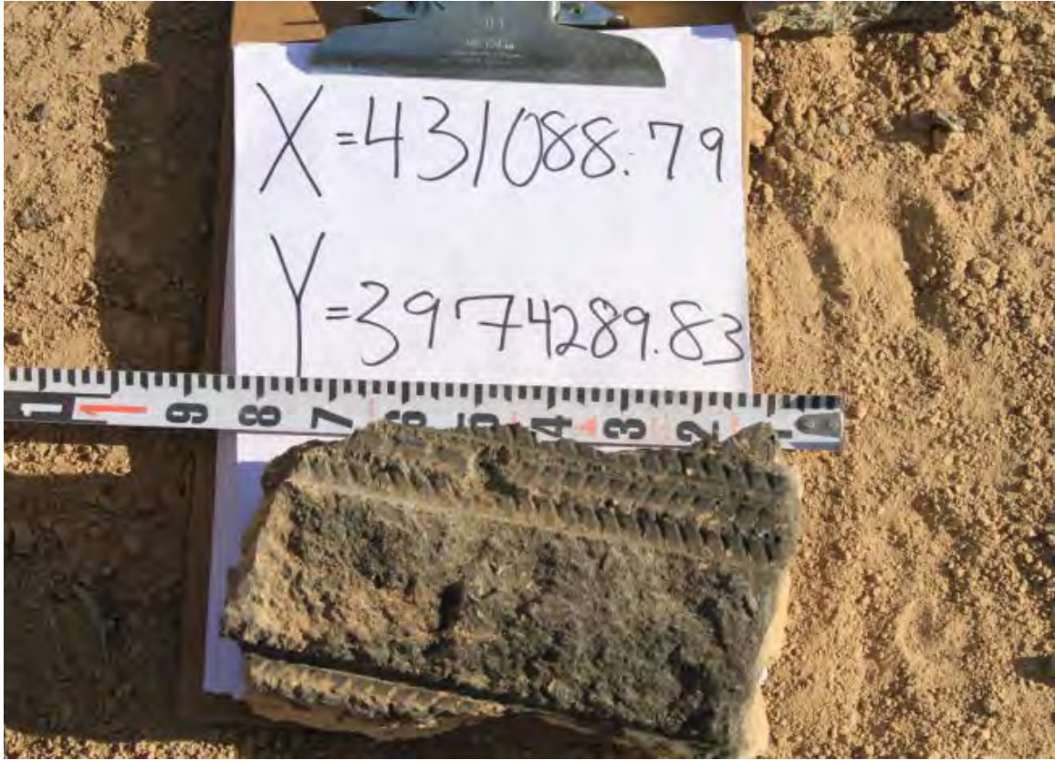
FIGURE III-G-17. Fragment That Weighed 2,925 g (Test 2). Note that the structure indicating where rebar had been located in the original undamaged concrete.
