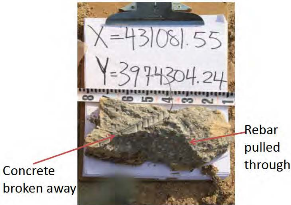
FIGURE III-40. Fragment Weighing 1,485 g From North Wall. Evidence of rebar pulled through the concrete during rupture, as well as concrete that was fractured around rebar exposing pattern of rebar and ribs.
