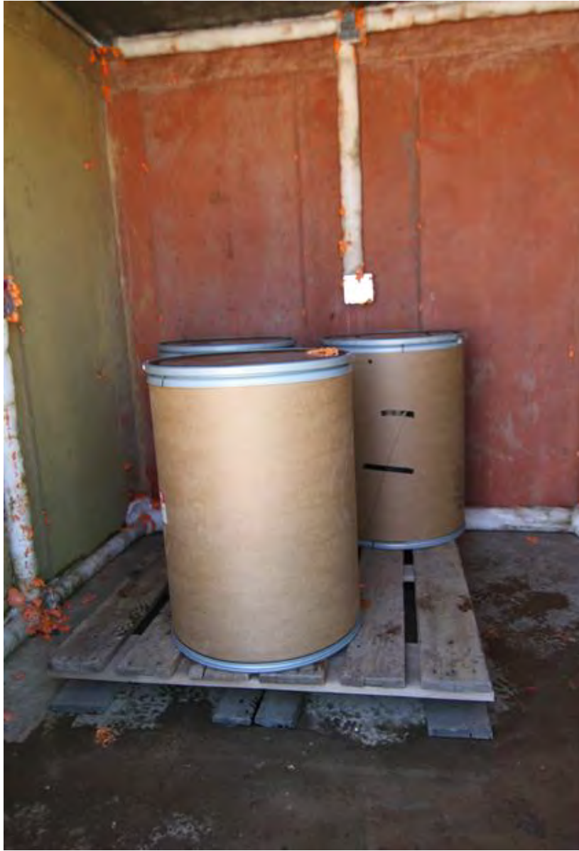
FIGURE II-1. Three Drums of M1 Propellant Placed Within the Structure for Test 1.
