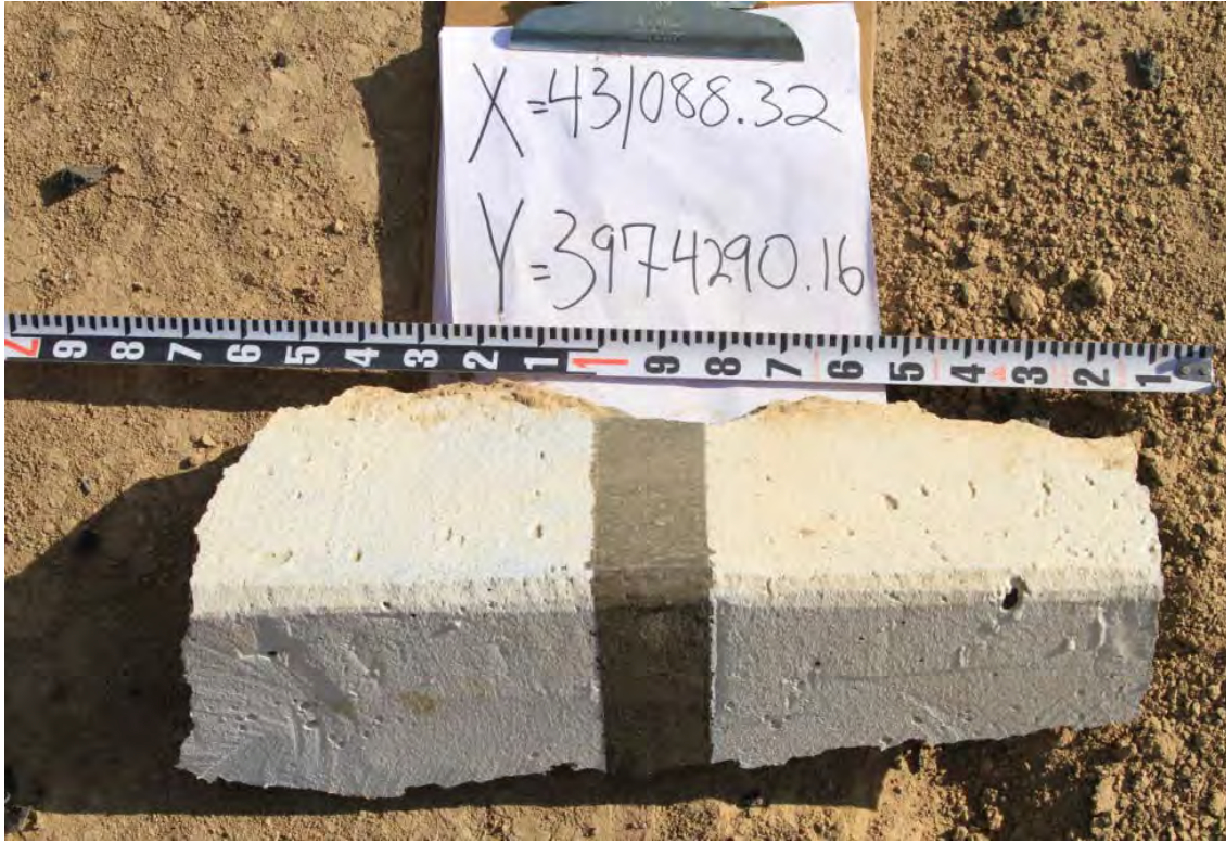
FIGURE III-G-5. Fragment Weighing 7,260 g Found Southeast of the Structure (Test 2).
