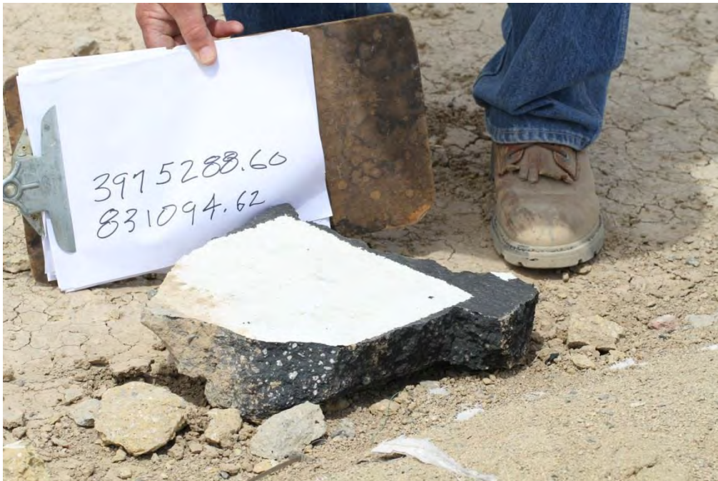
FIGURE V-G-5. Roof Fragment Weighing 8,740 g Found 14.25 m From Center of Original Structure (Test 4).
