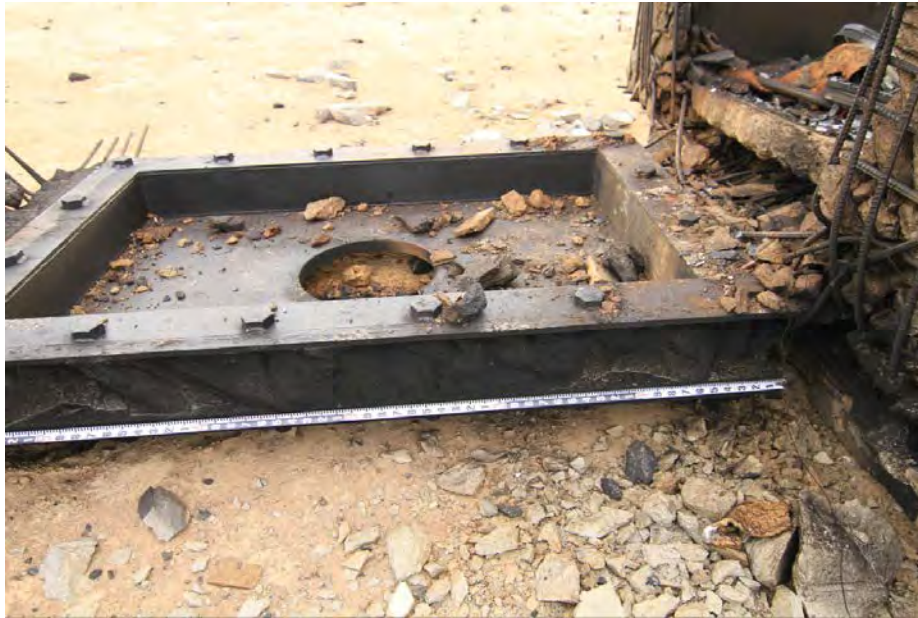
FIGURE III-23. Door Frame, Attached Plate With Orifice in Front of Structure (Test 2).
