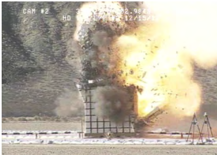
FIGURE III-17. Still Picture Taken From Video of Test 2 at Slightly Under 2 Seconds After Ignition, Showing Rupture of Structure and Resulting Fireball.
