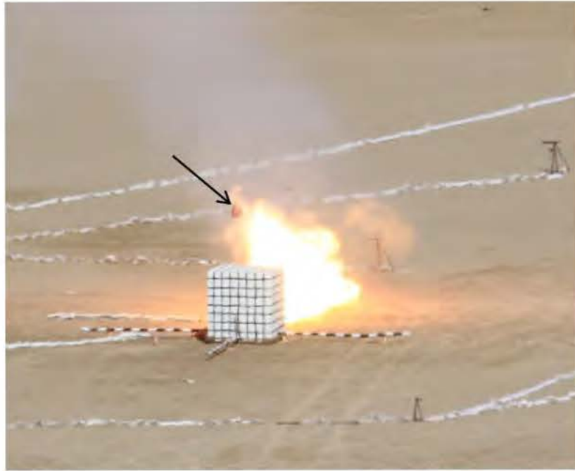
FIGURE IV-14. Structure and Plume of Test 3. At the left-hand side of the plume, a lid from one of the barrels can be seen.
