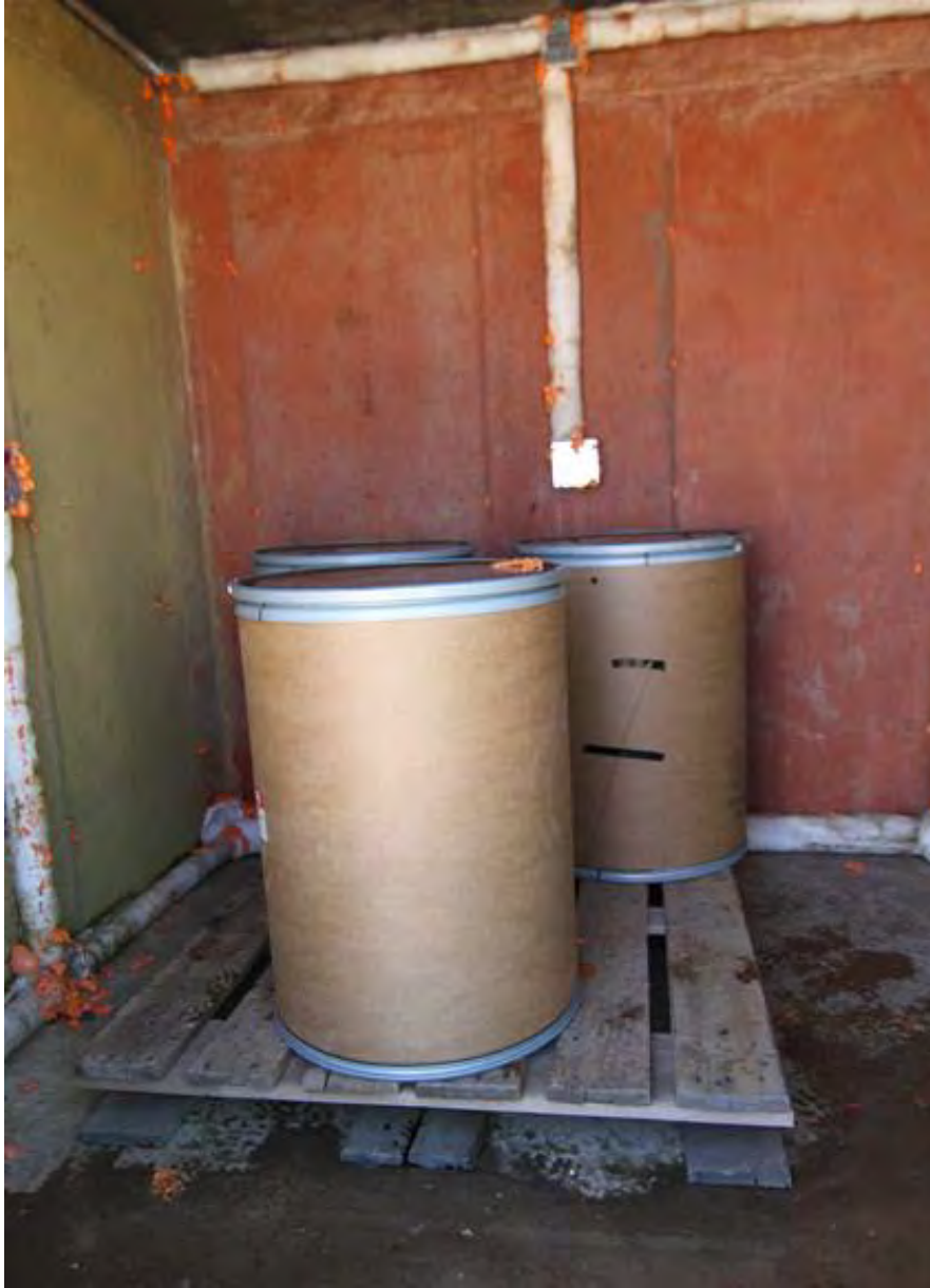
FIGURE I-6. Three Drums of M1 Propellant Placed Within the Structure for Test 1.
