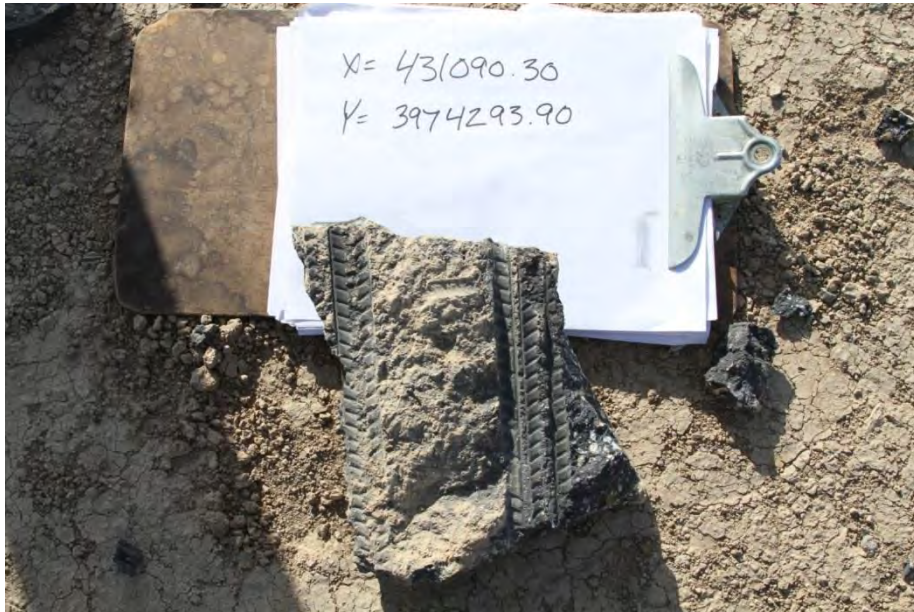
FIGURE V-G-16. Roof Fragment Weighing 3,535 g Found 7.6 m From the Center of the Structure (Test 4).
