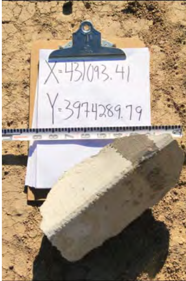
FIGURE III-G-15. One of Two Roof Fragments Found Adjacent to One Another Very Near to the Original Structure Site (Test 2). This fragment weighed 3,125 g.
