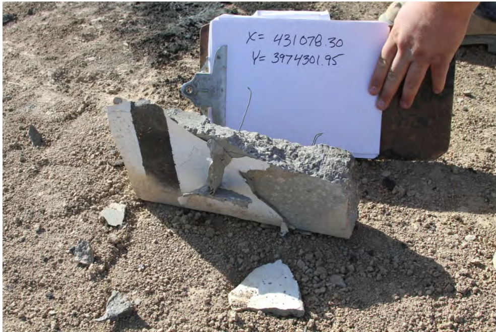
FIGURE V-44. Fragment From Front Wall Weighing 8,750 Grams and Found 17.5 Meters (57.4 Feet) FCOS (Test 4).
