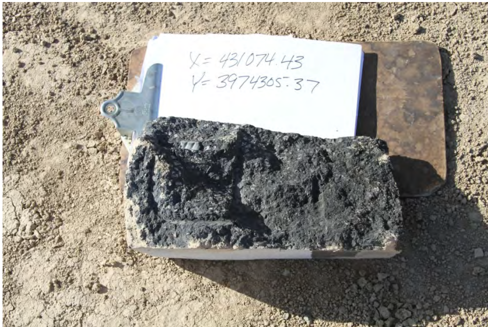
FIGURE V-43. Fragment From Roof Weighing 8,790 Grams Found 22.2 Meters (72.8 Feet) FCOS (Test 4).
