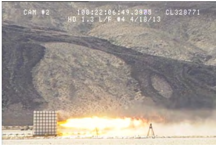
FIGURE V-18. Still Picture Taken From Video of Test 4 at 2 Seconds After Ignition Showing Plume Associated With Choked Flow.
