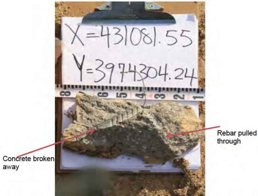
FIGURE III-G-23. Fragment Weighing 1,485 g From North Wall That Was Found 7 m North of North Wall (Test 2). Note the evidence for rebar being pulled through concrete on the right with perpendicular rebar impression with ribs indicating that the adjacent concrete fractured from rebar.
