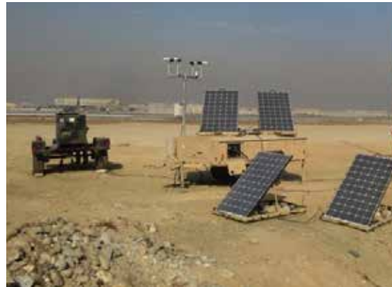
Weather stations powered by a 10kW Hybrid Solution.
