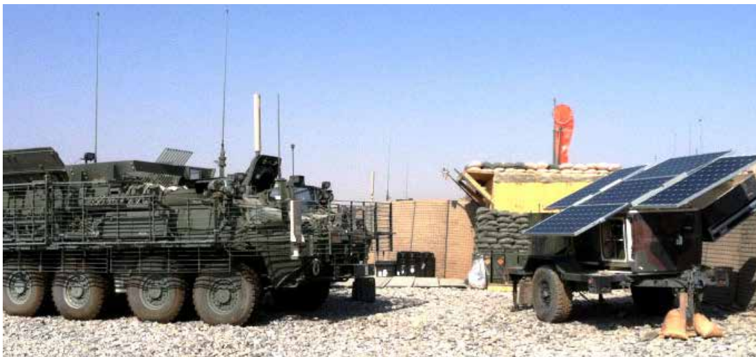
Solar panels at FOB being used to charge the batteries in a military vehicle.
