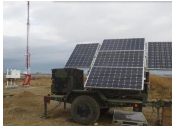
Weather station powered by a 5kW Hybrid Solution.
