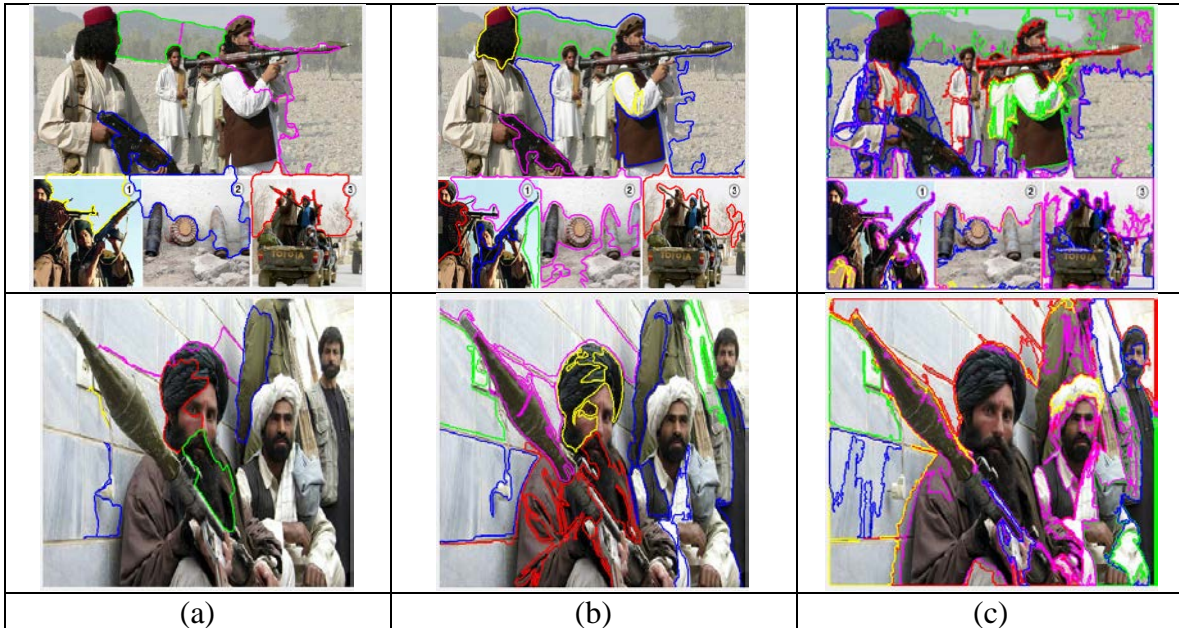
Figure 3: Segmentation results using the different segmentation algorithms. (a) Shows results of active contour model with image intensity driven external force field and automated initialization by Poisson inverse gradient, (b) shows segmentation results for image intensity and texture driven external force field with PIG based automated initialization. (c) Shows segmentation results using area morphological operators.
