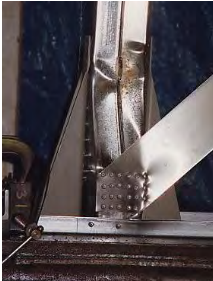
Figure 7-21. Bottom of left column of the A3c panel, showing column deformation and screw rotation.
