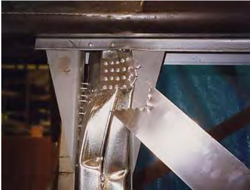
Figure 7-18. Close-up view of the A3a panel showing failed strap connection and column anchor.
