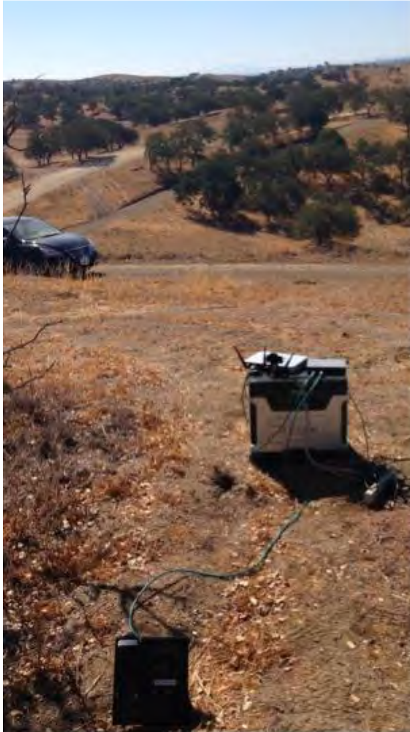
Deployment of the Cisco Rapid Response Kit 101 on day 3, August 13, 2014. This device allowed a phone for voice over IP to be connected. Also shown is Goal Zero battery.
