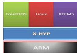
Figure 24. The Basic X-Hyp Architecture (from “X-hyp Paravirtualized,” n.d.)
