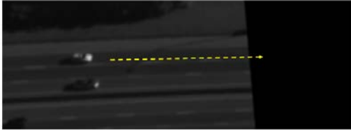
Fig. 7. Termination of tracks for targets leaving the working image boundary. predicted location is out of the working boundary, the tracker automatically terminates to avoid data access issues (Figure 7).
