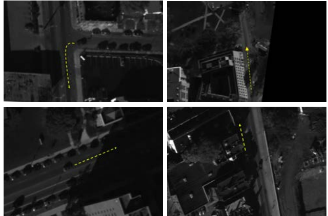
Fig. 8. Example of challenging conditions: Target appearance changes during turning (C4-1-0), low contrast and shadows (C3-3-4), shadow occlusion (C0-3-0) and combined building and shadow occlusion (C2-4-1) [49].
