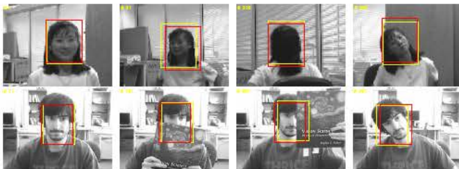
Fig. 12. Tracking results showing sample frames from 'girl' and 'faceocc2' sequences showing bounding boxes for ground-truth (yellow) and LoFT (red).
