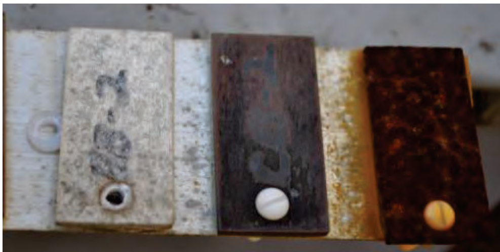
Figure A25. Rack 2, bare coupons at 24 months (photo 2). Note that this photo was taken after aluminum coupon was repositioned.
