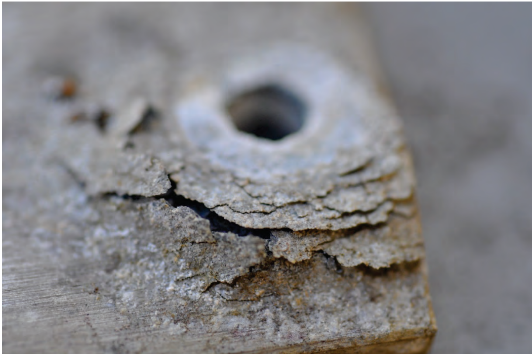
Figure 8. Exfoliation of a bare aluminum coupon after 24 months of on-site field exposure.
