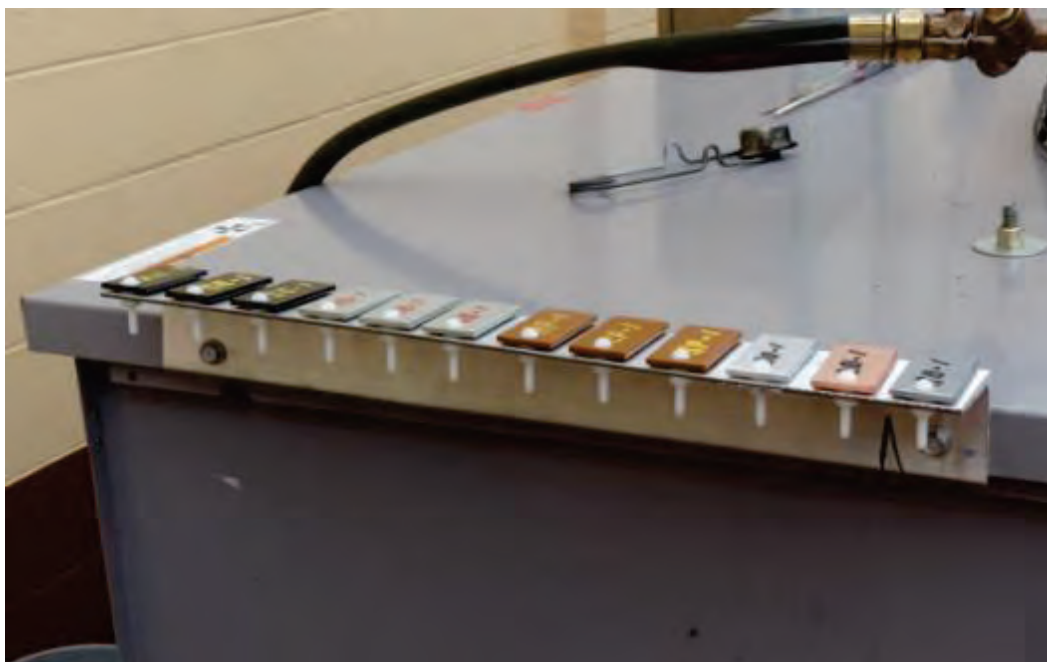
Figure 5. Aluminum coupon rack was fabricated to hold 12 coupons and mounted at each of the two condenser sites.
