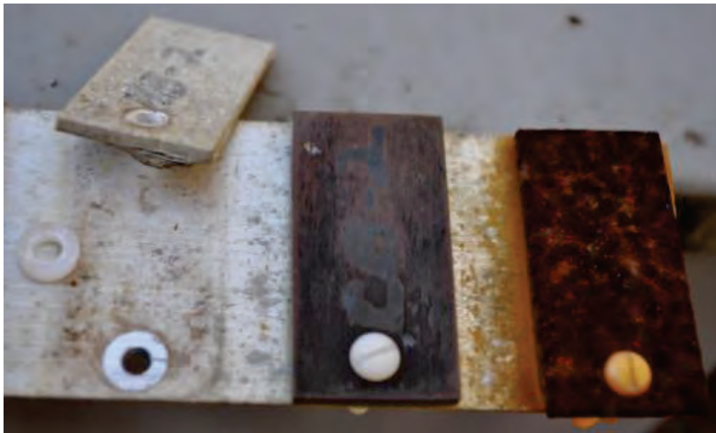
Figure A24. Rack 2, bare coupons at 24 months. Note that aluminum coupon (at far left) has become detached.
