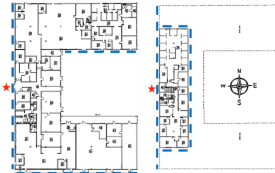
Figure 3. Floor plans for building (first floor is left, second floor is right). The red stars indicate the facade depicted in the photo; heavy dashed lines indicate facades that were retrofitted with dynamic windows
