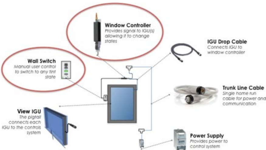
Figure 7. Dynamic window system. Controls are highlighted in red circles. The window controller determines automatic operation, while the wall switch allows direct user control.
