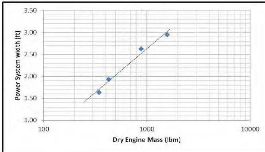
Figure 9. Power Plant Width Versus Dry Engine Mass
