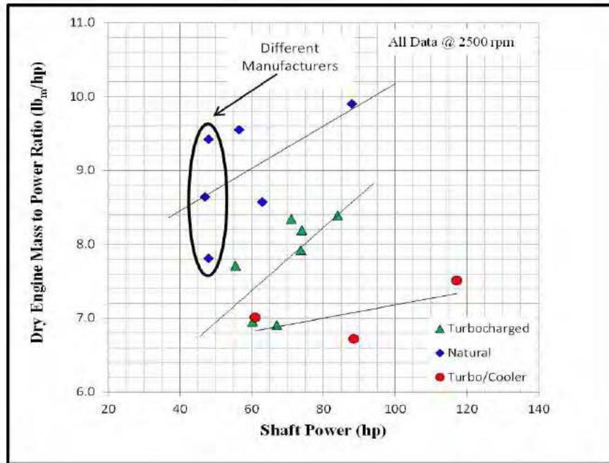
Figure 7. Power to Mass Ratio for Diesel Engines
