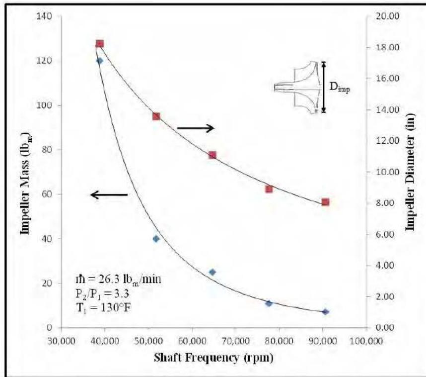
Figure 5. Impeller Characteristics (after Balje 1962; Xu and Amano 2012)
