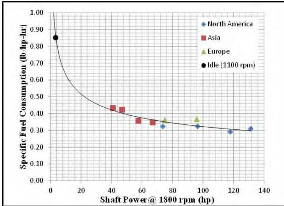
Figure 6. Specific Fuel Consumption Versus Shaft Power
