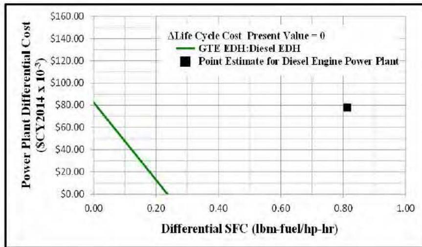
Figure 14. Equivalent ΔLCC GTE and Diesel EDH Architectures
