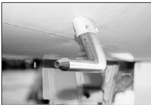
Figure 10-5. Typical Pitot Tube Installation, Underside Fuselage Without Integral Static Port
