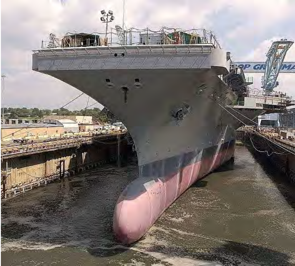
Figure 4. Bulbous bow installed on USS George H.W. Bush (CVN 77) (from Global Security 2014b).
