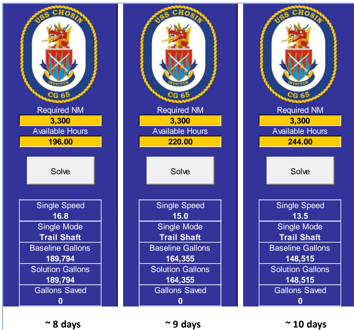
Figure 12. Fuel burned on a 3,300 nm transit in nine days +/- one day. A one day reduction in transit time will cause overburn of 25,439 gallons.
