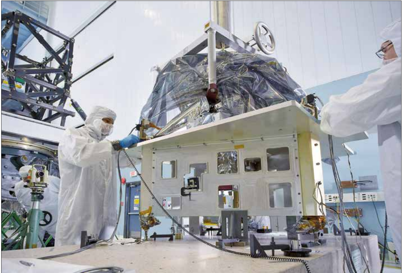
NASA's Mid-Infrared Instrument has camera and spectrograph that see light in mid-infrared region of electromagnetic spectrum (NASA/Chris Gunn/Rob Gutro)
