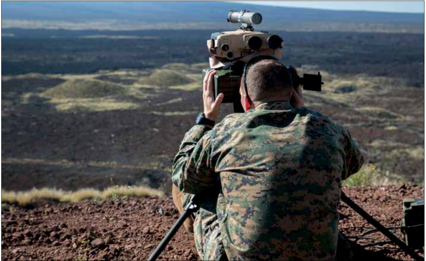
Joint terminal attack controller sights target with AN/PED-1 Lightweight Laser Designator Rangefinder to mark simulated hostile threats for air assets (U.S. Marine Corps/Devon Tindle)
