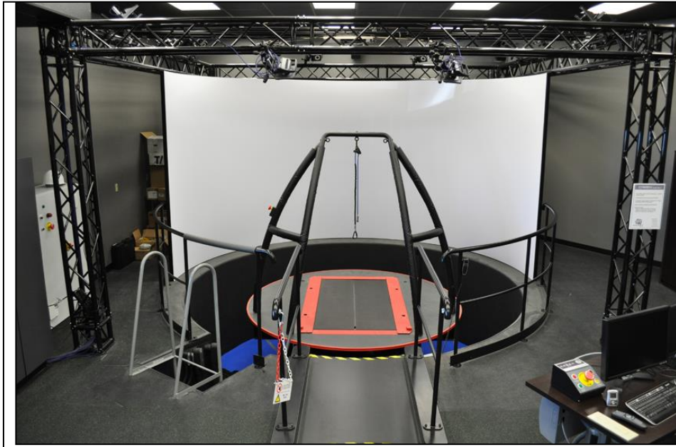
Figure 1. Computer Assisted Rehabilitation Environment (CAREN).
