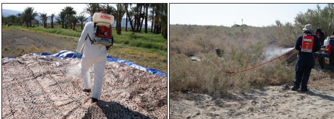
Fig. 6-6. Treating ULCANS camo netting with Demand CS residual \lambda -cyhalothrin using a Stihl SR 450 backpack sprayer (left), and treating desert vegetation with Talstar bifenthrin using an Electroton electrostatic backpack sprayer (right) at experimental plots in southern California. Photos: (L) Seth Britch, USDA; (R) Wayne Wynn, USDA.
