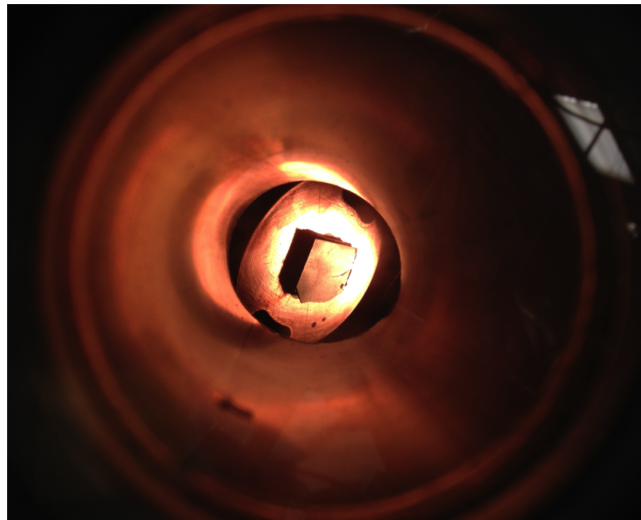
Figure 27. Photograph of indium target and tungsten converter mounted on the copper cold head in the evacuated Dynamitron target chamber.
