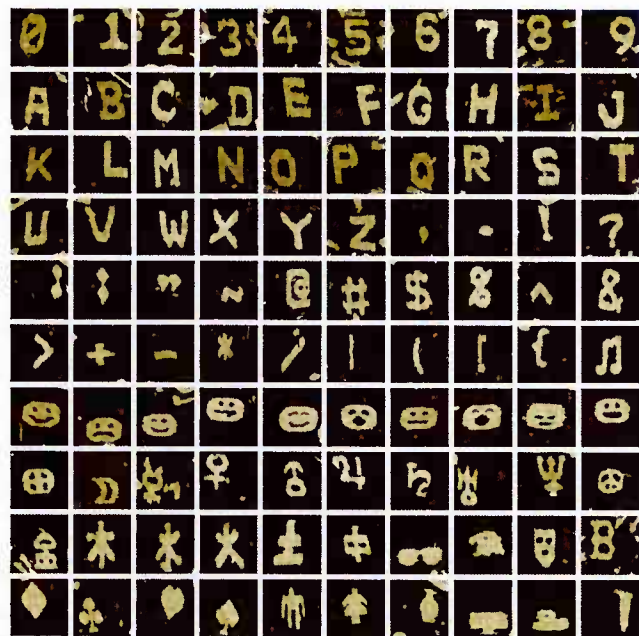
Figure 4 | Complex shapes designed using a molecular canvas. AFM images of 100 distinct shapes, including the 26 capital letters of the Latin alphabet, 10 Arabic numerals, 23 punctuation marks and other standard keyboard symbols, 10 emoticons, 9 astrological symbols, 6 Chinese characters and various miscellaneous symbols. Each image is 150\text{ nm} \times 150\text{ nm} in size.
