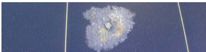
Figure-23: Corrosion of PV material due to a pin-size hole at Site II (NAS Patuxent River).
