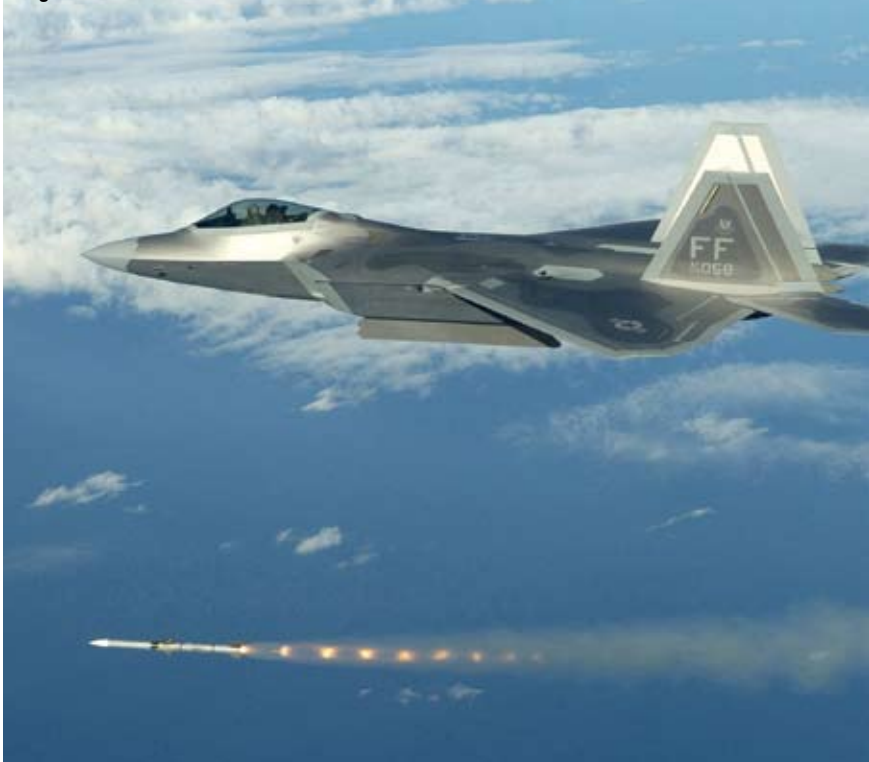
F-22A Raptor fires AIM-120 advanced medium-range air-to-air missile at aerial target drone over Gulf of Mexico
