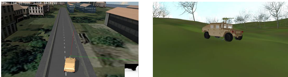
Figure 1: HMMWV UGV simulator: The image on the left depicts an urban driving scenario which exercises the vehicle's autonomous way-point and road following software. The image on the right shows the same vehicle in an off-road scenario with obstacle avoidance capability.
