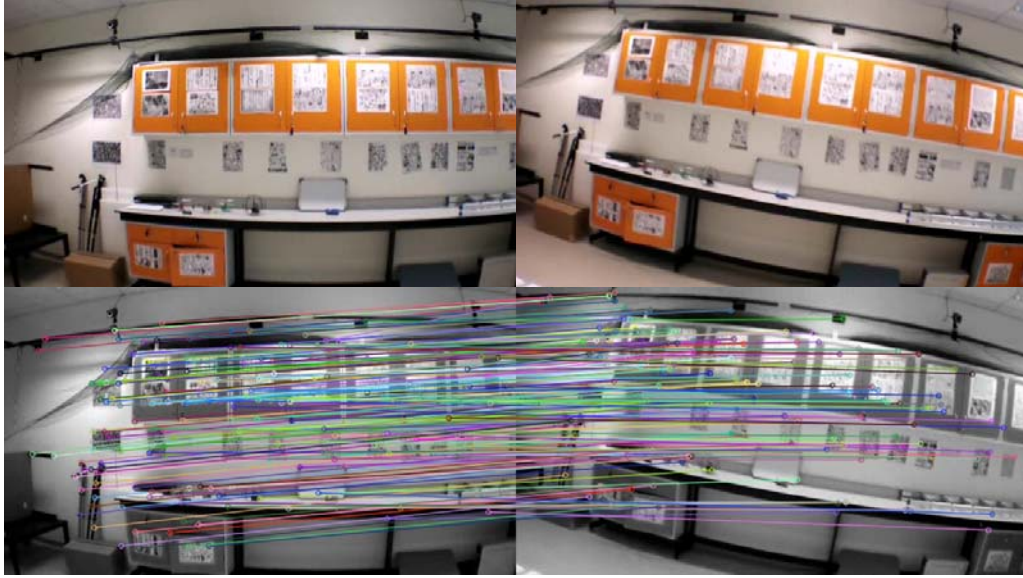
Figure 5. The left is the found key frame and the right is the current image. 215 feature correspondences are found to re-localize the camera.
