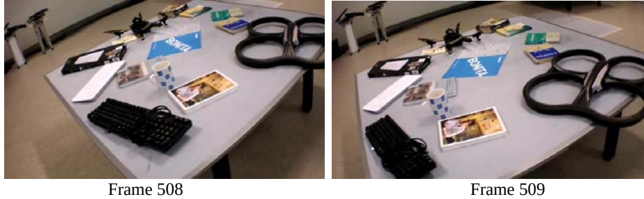
Fig.2. Two consecutive images captured by a camera on a UAV. Some frames are lost obviously due to the wireless transmission and the view point is changed significantly, which causes feature tracking failure.
