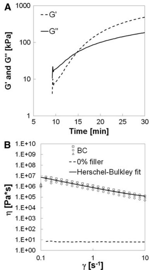
**FIG. 1.** Rheological properties of the biocomposite (BC) measured by rheometry. **(A)**  $G'$  represents the storage modulus and  $G''$  the loss modulus. The  $G'$   $G''$  crossover point is assumed to be the working time of the BC. **(B)** Viscosity versus shear rate plot illustrating calculation of the yield stress using the Herschel Bulkley model.
