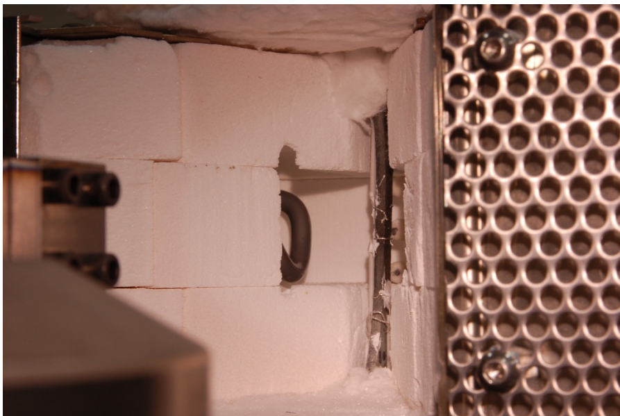
Figure 16. Mellen furnace with thermal profile specimen installed
