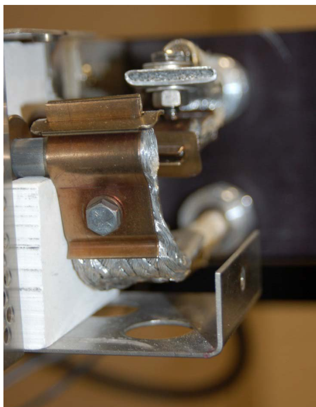
Figure 11. End view of alumina block furnace element support
