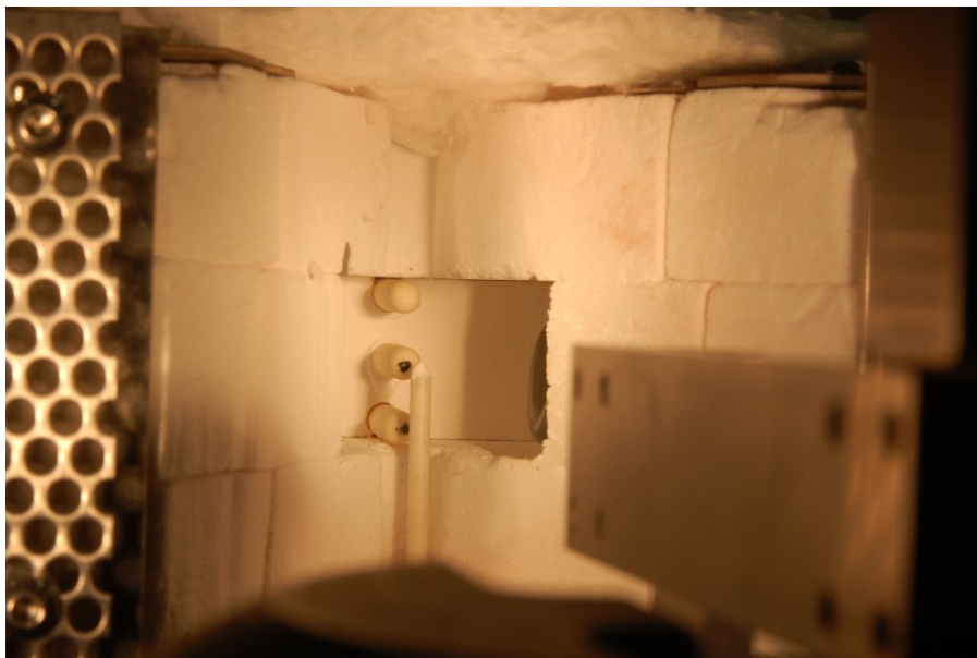
Figure 20. Single ceramic TC probe positioned at furnace centerline
