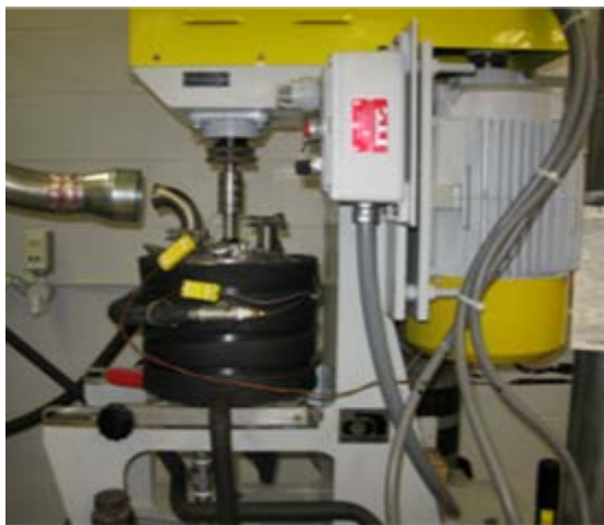
Fig. 1 The Szegvari attritor available at the US Army Research Laboratory (ARL), modified to enable cryogenic attrition
