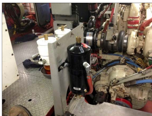
Figure 2. RCI fuel purifier installed on starboard Racor mount.
