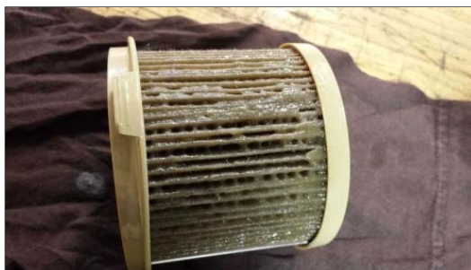
Figure 7. B100 gel on a Racor filter.
