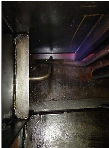
Figure 4. Stripped starboard fuel tank and pickup pipe.
