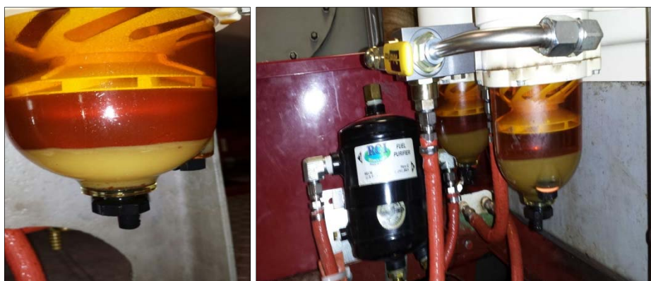
Figure 6. B100 completely separated in the oil-water separator.
