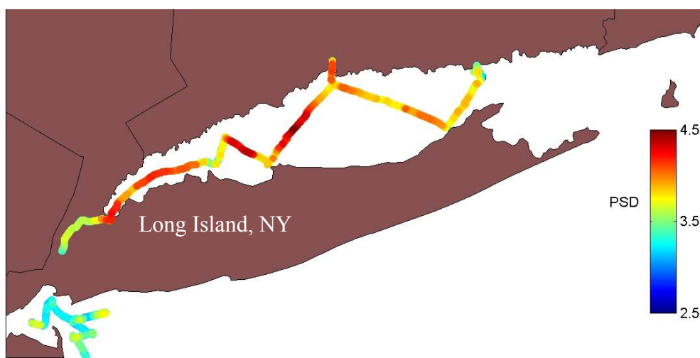
Fig. 4. Slopes of the particle size distribution in Long Island Sound measured with the LISST instrument are high relative to Hudson River plume indicating a prevalence of small highly backscattering particles.
