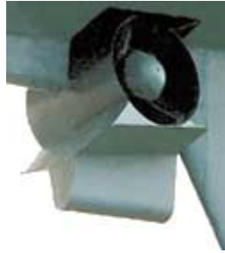
Figure 35 – Extendable bow thruster with moving keel piece
