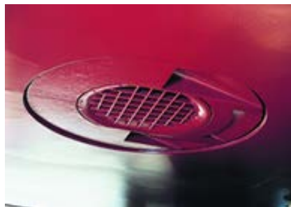
Figure 37 – Pump jet integrated with a ship's hull
