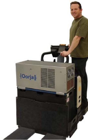
Figure 70 – Material handler powered by an Oorja DMFC
