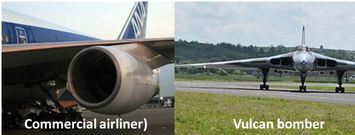
Figure 25 – Sponsoned versus integrated engines
