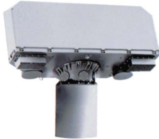
Figure 11: Sea GIRAFFE AMB's 3-D phased array antenna assembly (from [15])
