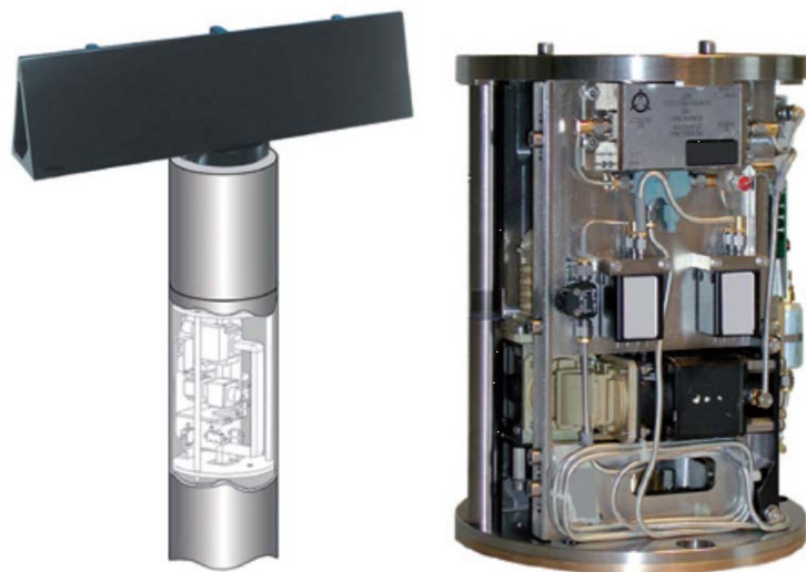
Figure 19: Transceiver unit from which fits in a submarine mast (from [23])
