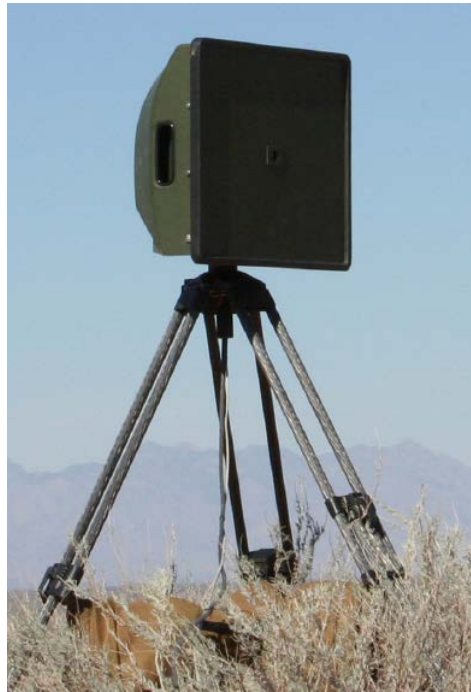
Figure 23: Squire Radar Antenna (from [31])
