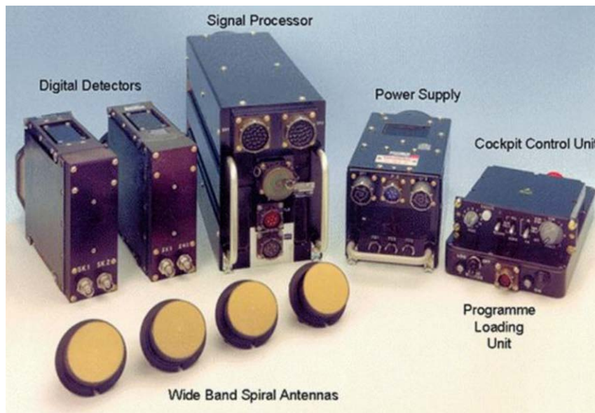
Figure 59: SEER RWR System Components (from [79])
