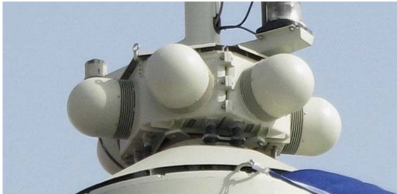
Figure 73: SEAL on mast of Abu Dhabi-class FHS of the UAE Navy (from [99])
