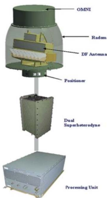
Figure 49: ELINT-FD Narrow-band ELINT System Schematic (from [67])
