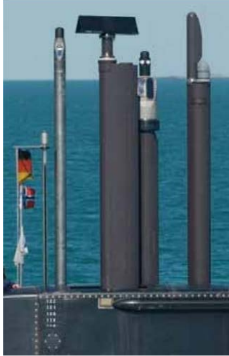
Figure 67: UME-100 System installed onboard South African Navy Type 209 submarine (from [87])
