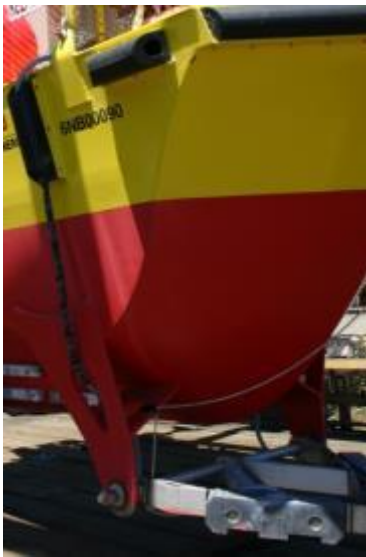
Figure 35: Bow load cell cable routing along the yoke and hull (Hellin 2013-a).
