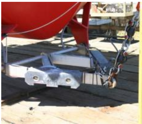
Figure 52: Yoke secured in the “up” position (Hellin 2013-a)
