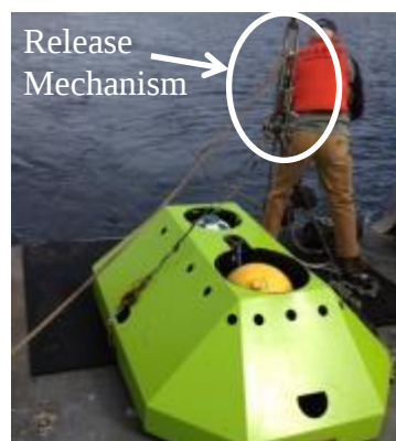
Figure 63: AWAC rigged for deployment
