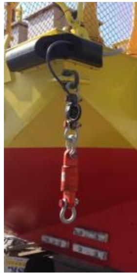
Figure 36: Port load cell cable routing (Moran 2013).
