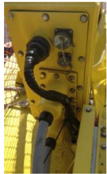
Figure 37: Junction box with watertight gland (Moran 2013).
