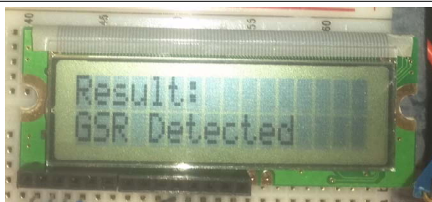
Fig. 12. Electronic readout for GSR sample on bread boarded GSR screening tool.
