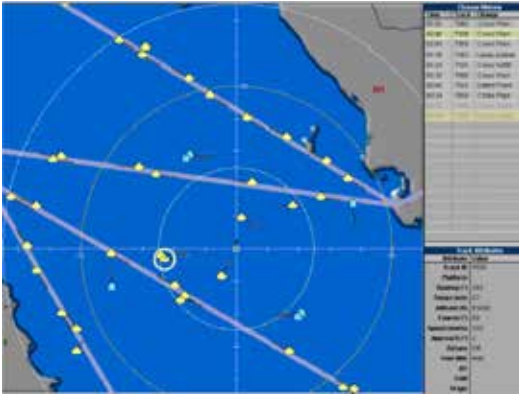
Fig. 5. Interruption recovery aid—textual event history list (CHEX—upper right) (adapted from [116], with permission).
