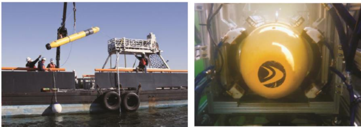
Figure 9: Battelle-developed Docking Station for Bluefin 21 AUV
