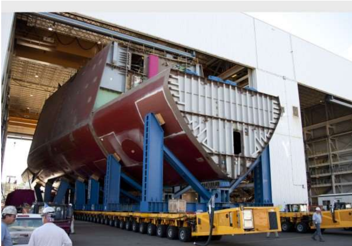
Figure 31. Ultra Unit section of DDG-1000.
