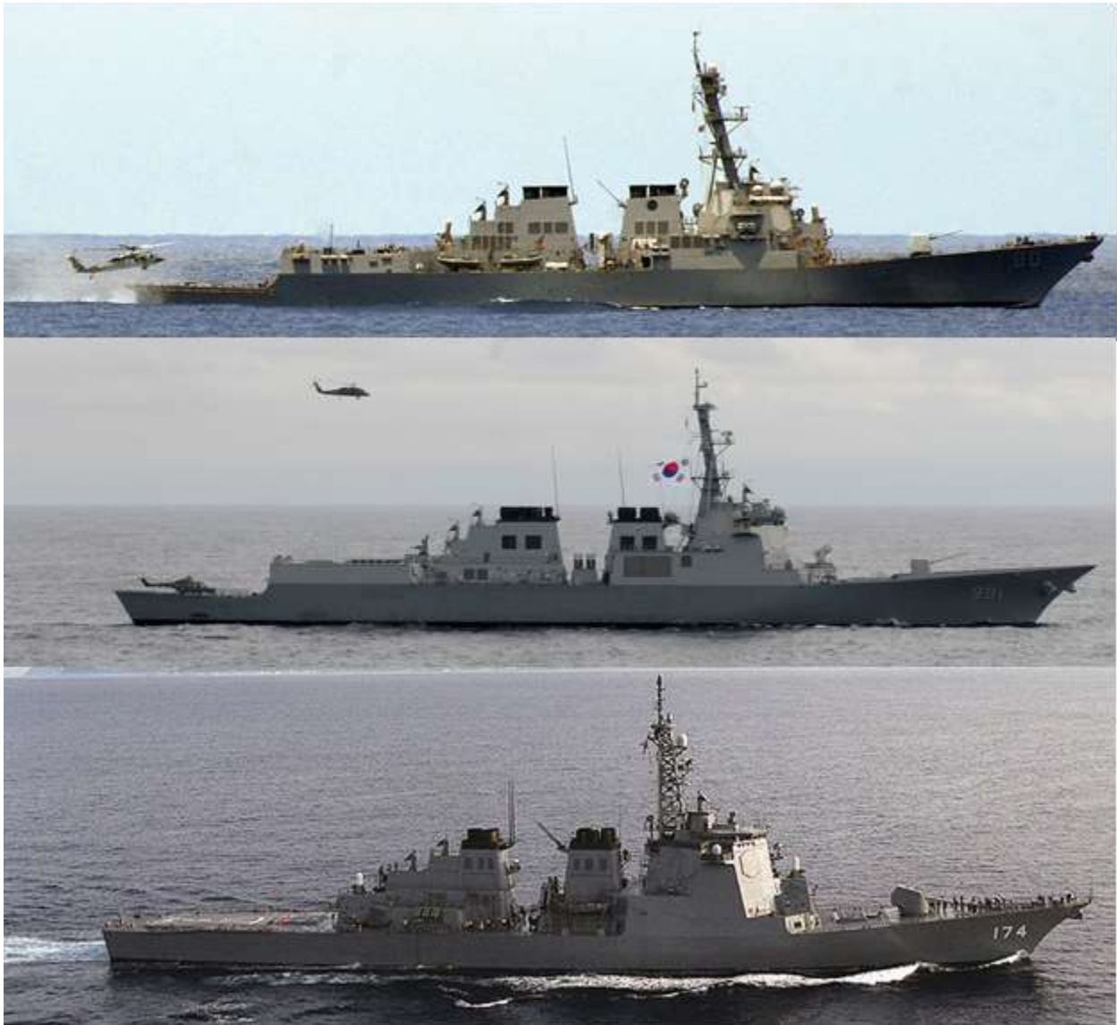
Figure 14. Top – US Arleigh Burke Destroyer (DDG-80) Middle – South Korean KDX-III Destroyer (DDG-991) Bottom – Japanese Kongo Class Destroyer (DDG 174)
