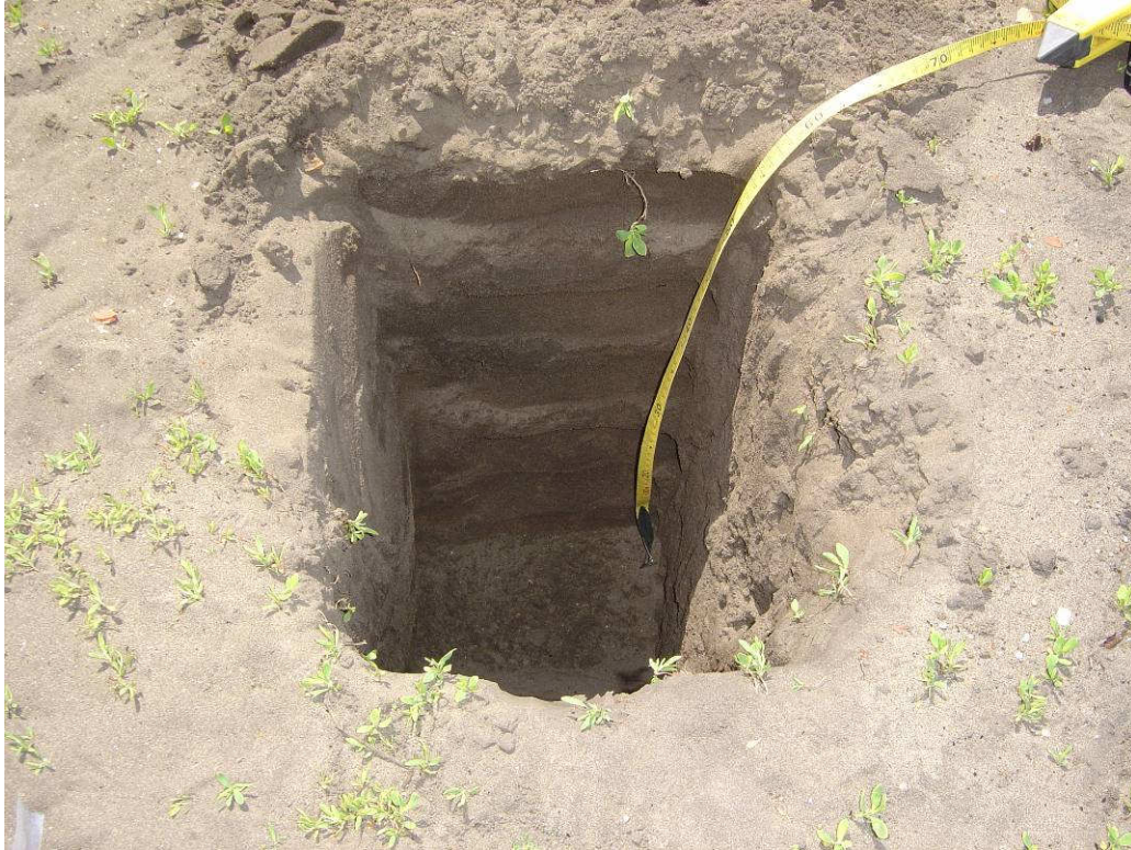
Figure 22. Vertical sampling in one of two holes 60-cm deep at the firing point in Range 22.
