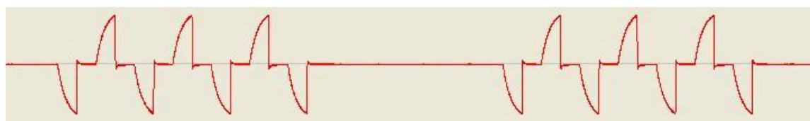
Figure 31: EM63 waveform – At 50 Hz powerline setting and H frequency, repetition frequency of the waveform is at 30 Hz while turned on – 8.333 msec +/-off/-off
