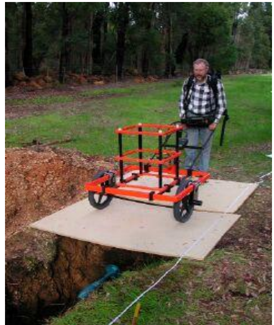
Figure 10 – BEAMOD™ Mk.1 prototype system (left) and EM63 (right) used over the EMIT test pit, Mundaring, Western Australia
