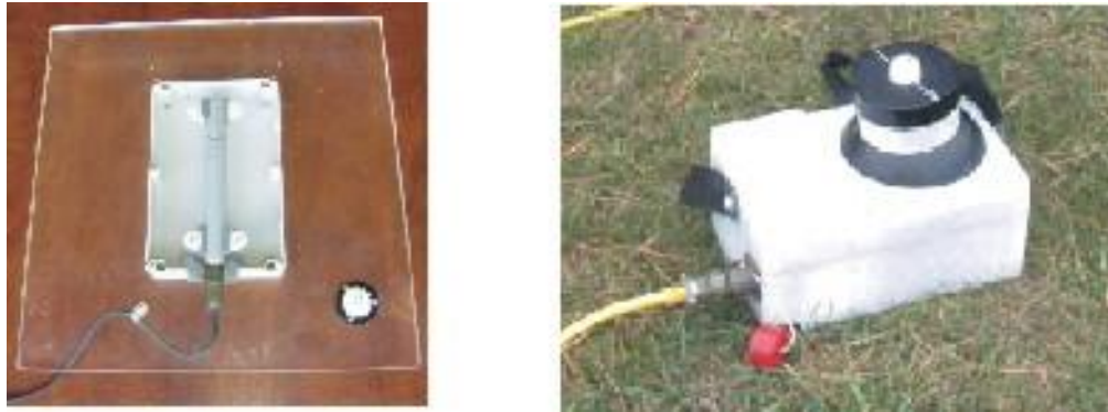
Figure 1 – Pictures of Bartington fluxgate magnetometer (left) and CSIRO SQUID magnetometer (right)
