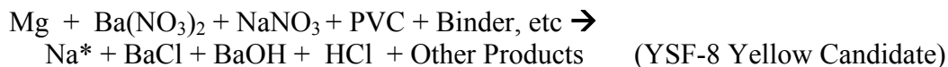
Figure 9. General Reaction Pathways for Existing and Perchlorate-Free Red, Green and Yellow Signal Flare Compositions
