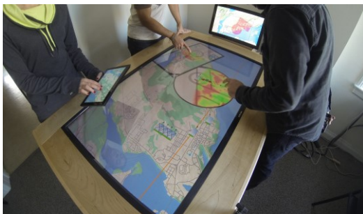
Figure 1. OrMiS supports military simulation and C2 by allowing small groups of people to collaborate around a shared touch surface. OrMiS is based on a large multi-touch table, handheld tablets, and a radar view display.
