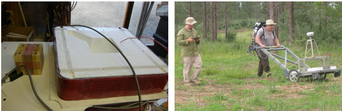
Figure 2-1 – Individual TEMTADS/3D EMI sensor with 3-axis receiver under construction.
