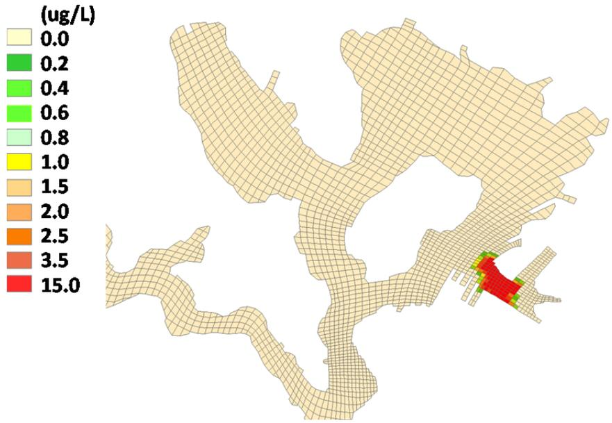
Figure 75. Initial silt-particle-bound copper concentrations at surface layer for CH3D fate and transport simulation at  $t = 0$  after resuspension from prop wash (color key applies to Figure 75–59, respectively).
