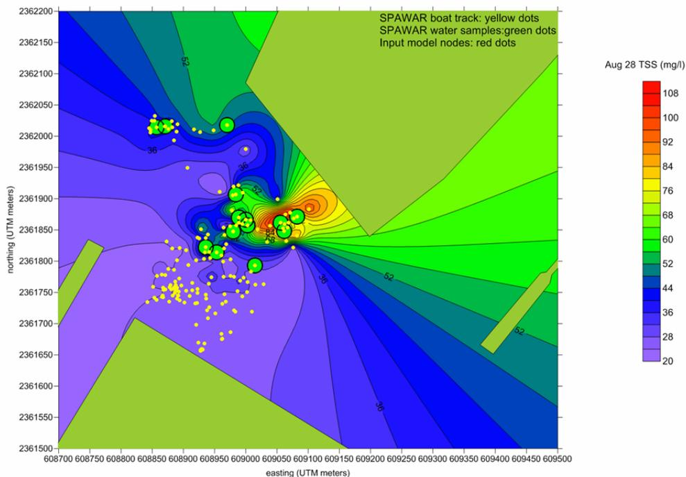
Figure 61. Locations for water samples, OBS data, and ADCP backscattering data for Bravo Pier, Pearl Harbor.
