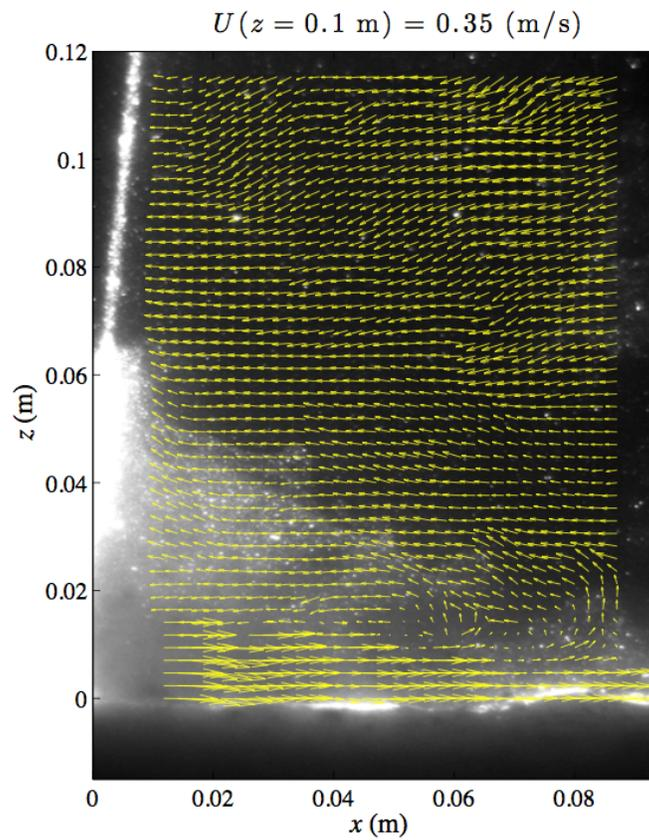
Figure 20. Sample PIV image: initiation of sediment resuspension.
