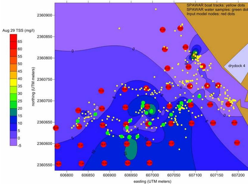
Figure 50. Model cells with the initial plume loads (red circles) estimated and extrapolated (e.g., color contours for TSS) from the measured water samples (green circles) and OBS data (yellow circles) for Oscar Pier.
