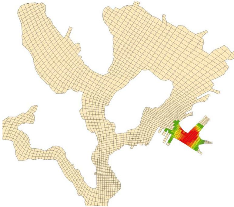
Figure 79. Simulated silt-particle-bound copper concentrations at bottom layer at  $t = 3$  hours after prop-wash resuspension.
