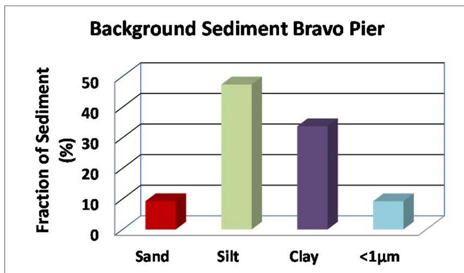
Figure 58. Water column particle size fractions and background sediment for clay (.4 to 5 µm), silt (5 to 60 µm) and sand (> 60 µm) for Bravo Pier in Pearl Harbor.
