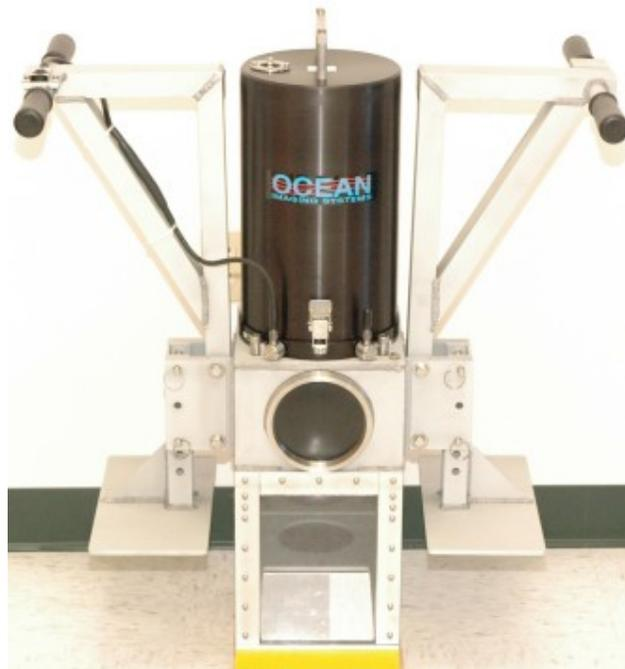
Figure 37. The hand-held, diver-deployed sediment profile camera used in Pearl Harbor.
