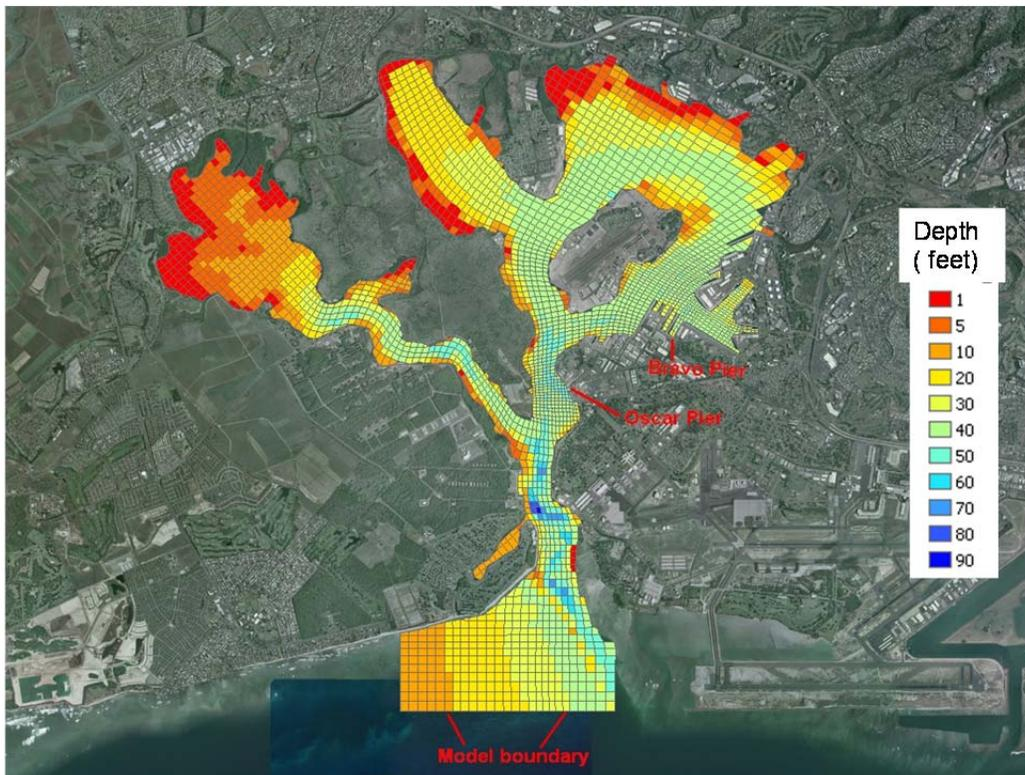
Figure 46. Refined fate and transport model, CH3D, for Pearl Harbor.
