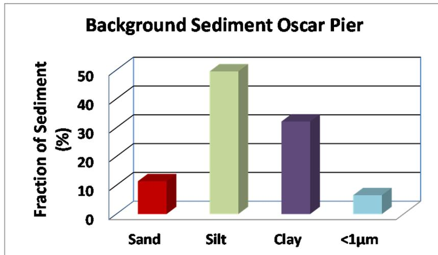
Figure 59. Water column particle size fractions and background sediment for clay (0.4 to 5.0 µm), silt (5 to 60 µm) and sand (> 60 µm) for Oscar Pier in Pearl Harbor.
