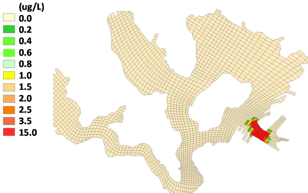
Figure 69. Initial dissolved copper concentrations at surface layer for CH3D fate and transport simulation at t = 0 after resuspension from prop wash (color key applies to Figure 69 through Figure 74, inclusive).
