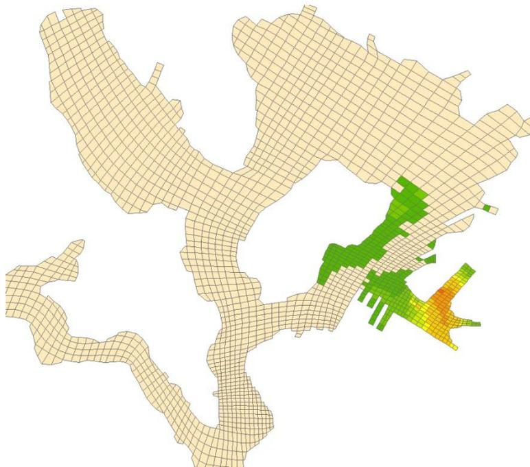
Figure 80. Simulated silt-particle-bound copper concentrations at bottom layer at  $t = 9$  hours after prop-wash resuspension.
