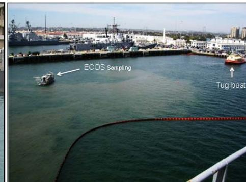
Figure 4. Diagram and views of the resuspension event procedure, including the tug-boat-induced bottom sediment resuspension, sampling of the plume, and mapping track on the plume.
