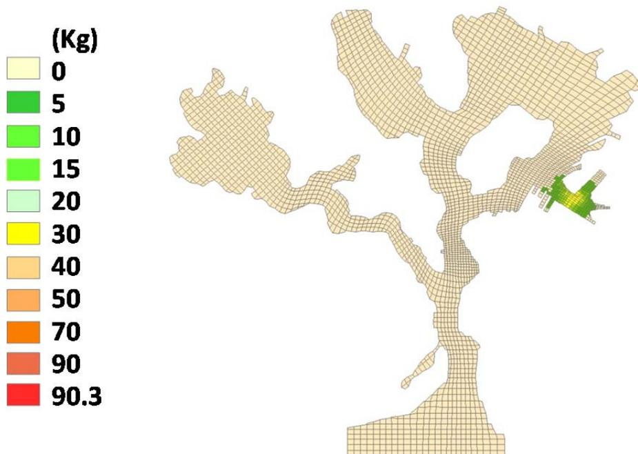
Figure 84. Simulated silt-particle-bound deposits to the bottom bed at t = 3 hours after prop-wash resuspension (color key applies to Figure 84–Figure 88, inclusive).
