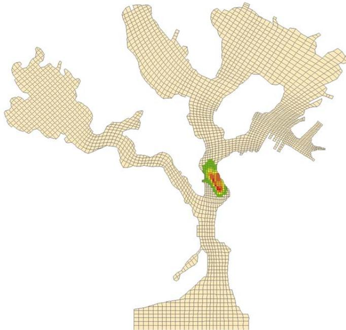
Figure 89. Initial dissolved copper concentrations at Oscar Pier surface layer for CH3D simulation at t = 0 after resuspension from prop wash (color key applies to Figure 89–Figure 99, inclusive).
