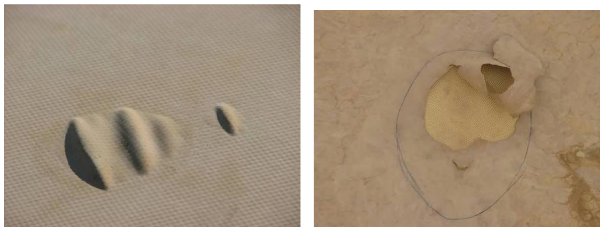
Figure 2. Fabric blistering due to hydrolysis.
