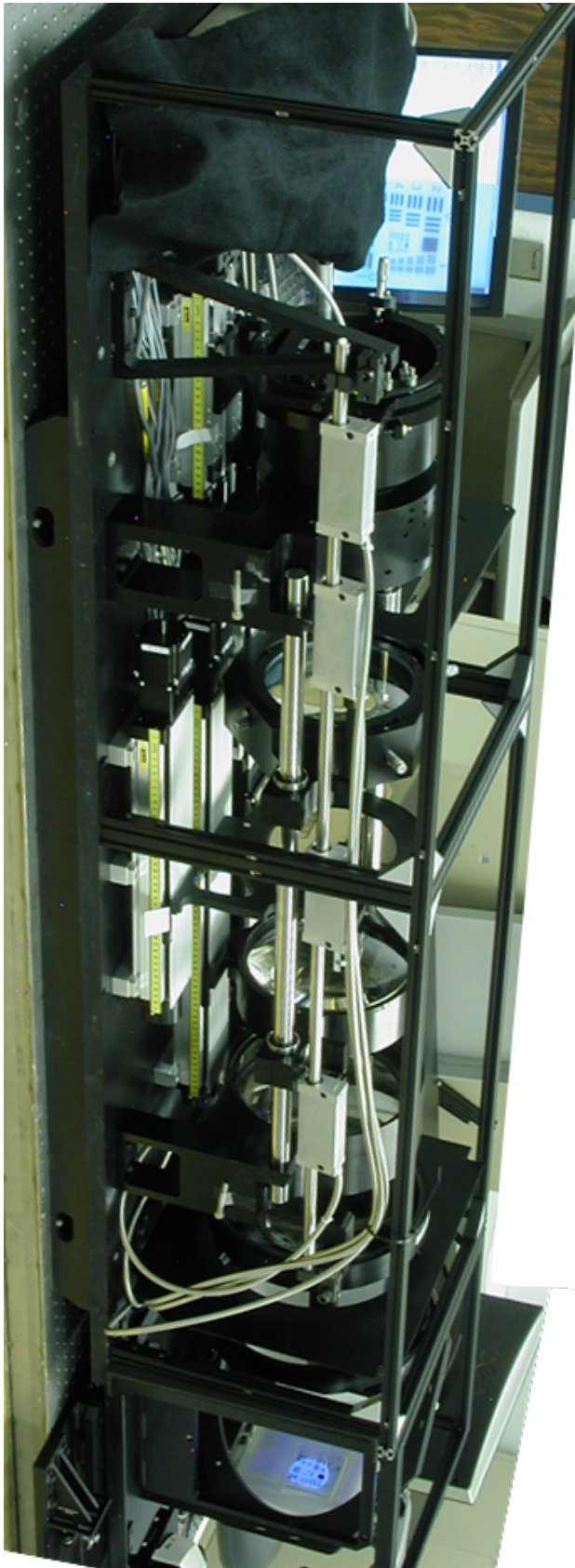
Figure 7. The first zoom lens assembly.
