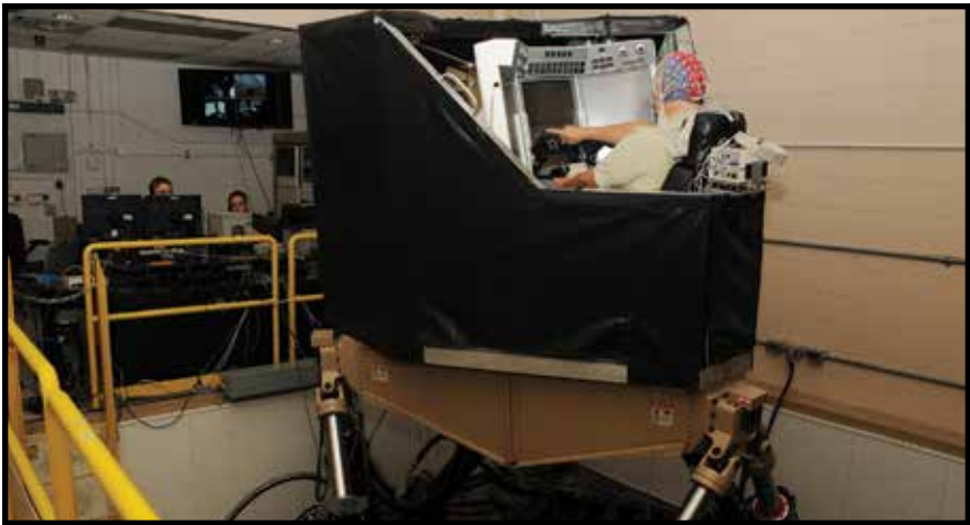
FIGURE 6. US ARMY TANK AUTOMOTIVE RESEARCH, DEVELOPMENT AND ENGINEERING CENTER (TARDEC)’S RIDE MOTION SIMULATOR (RMS)
