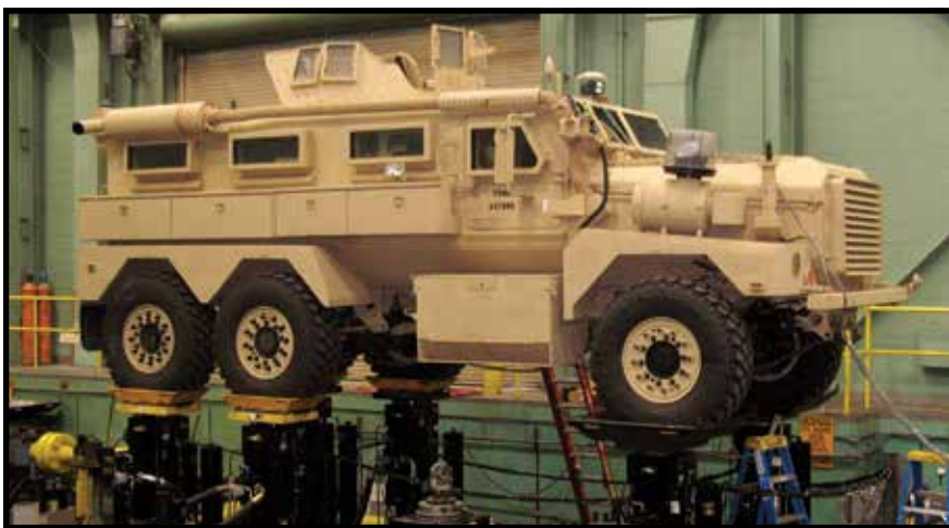
FIGURE 7. US ARMY TARDEC’S N-POST SHAKER
