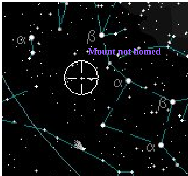
Figure 35. TheSky interface during b-type mount failure
