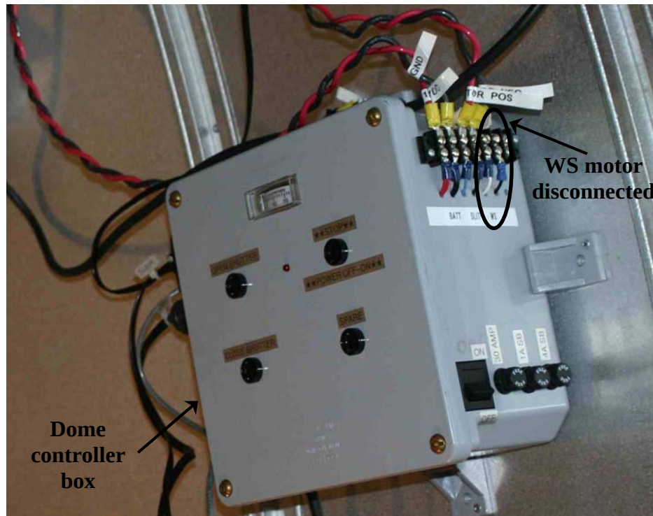
Figure 31. WS motor disconnected from the dome controller box
