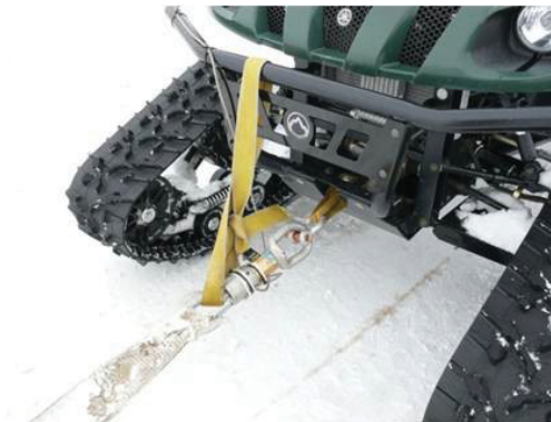
(b) Load cell on towed vehicle.
