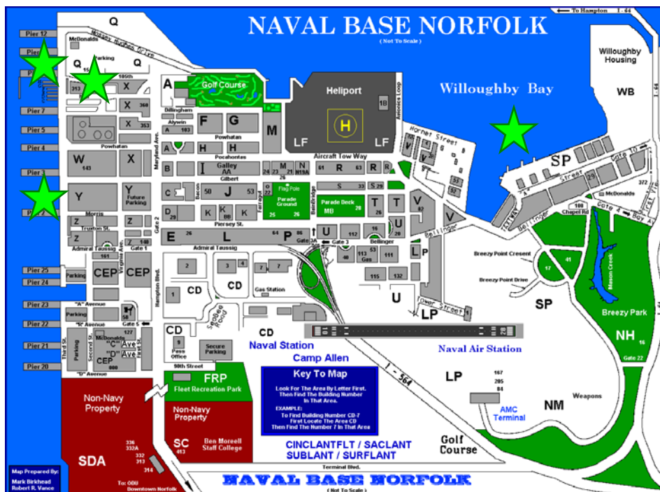
Figure 3.5 Location of Spill Sentry sensors at NAVSTA Norfolk. (Sensor and base-station locations are shown as green stars).
